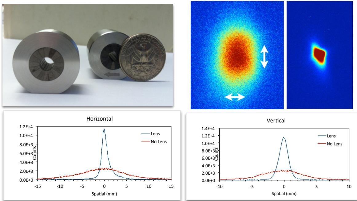
**Figure 1: Electron beam transport.** Left shows the compact permanent-magnet quadrupole lenses. The unfocused electron beam is shown in the middle and the collimated beam on the right. The white arrows indicate a 5 mm size corresponding to a solid angle of 2.9 mrad. Horizontal and vertical line-outs of the unfocused (collimated) electron beam are shown on the bottom.
