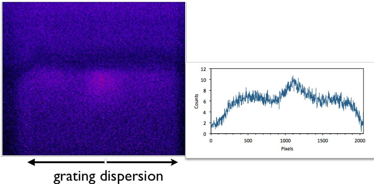
**Figure 3: Observed undulator spectrum.** Left shows the observed undulator radiation signal measured with the transmission grating-based X-ray spectrometer. The bright spot is the zeroth diffraction order (transmitted beam). The lineout on the right shows the signal of the  $\pm 1^{\text{st}}$  diffraction orders.
