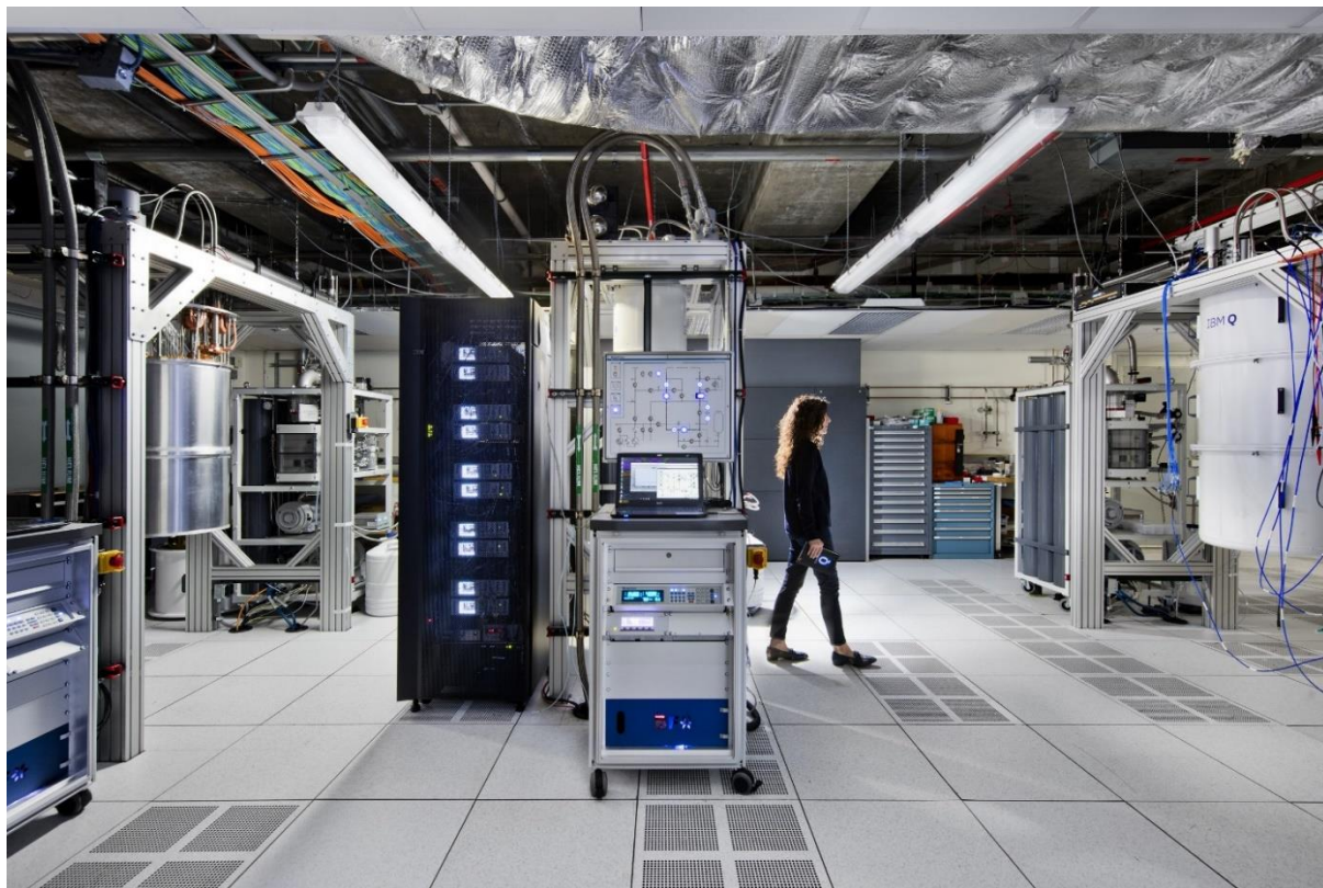
Figure 5: IBM's quantum computing center at the Thomas J. Watson Center in Yorktown Heights, New York. The center holds quantum computers in huge cryogenic tanks (far right) that are airconditioned to a fraction of a degree above absolute zero (photo credit: IBM, Feb 2018).
