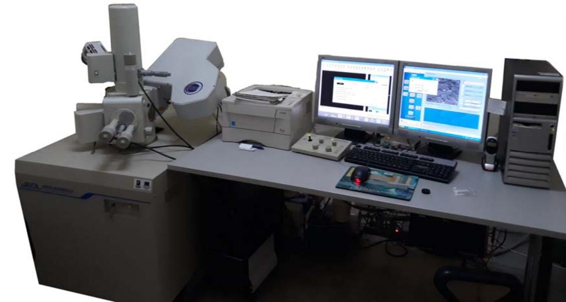
**Figure 11:** Scanning electron microscope (Jeol JSM – 6390LV) employed in the microstructure investigation.
