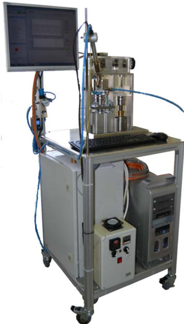
**Figure 4:** Experimental set-up for thermal fatigue tests at constant force through a pneumatic piston.
