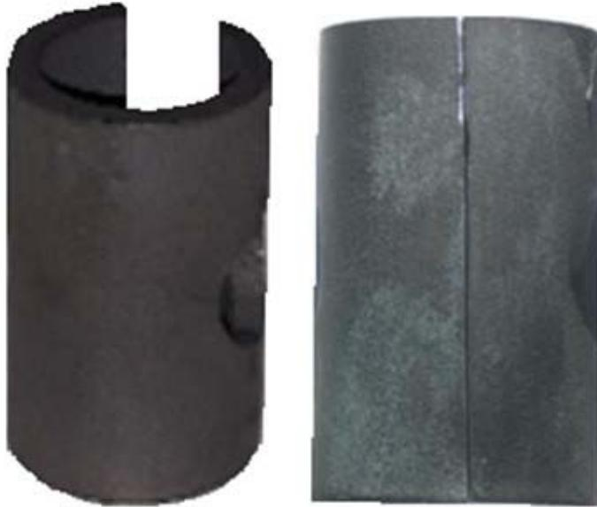
**Figure 41:** Outer surface of the uncleaned specimen before and after the combined corrosion and fatigue experiment.
