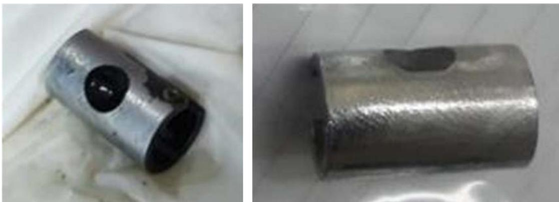
**Figure 30:** The specimen parent alloy which was revealed from electrochemical cleaning.
