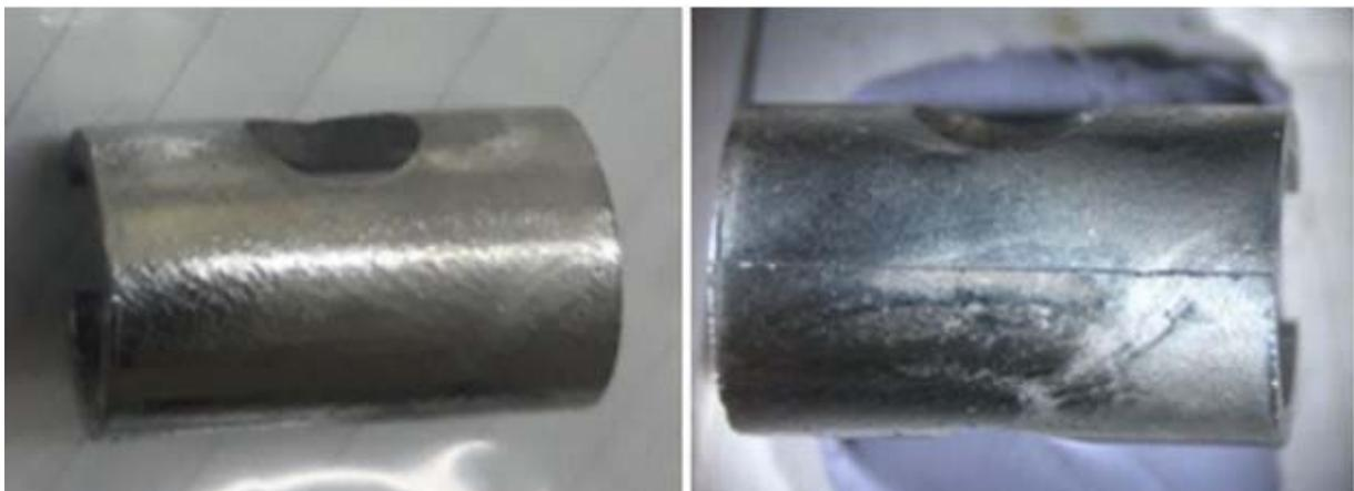
**Figure 33:** Outer surface of the cleaned specimen before and after the corrosion-fatigue experiment.
