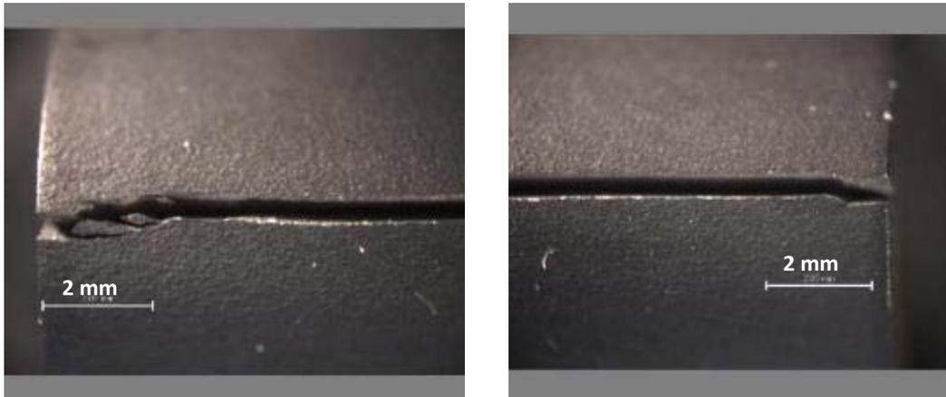
**Figure 25:** Fractured surface of the specimen of the 1<sup>st</sup> combined corrosion and fatigue experiment. Right image: beginning of the crack. Left image: end of the crack.
