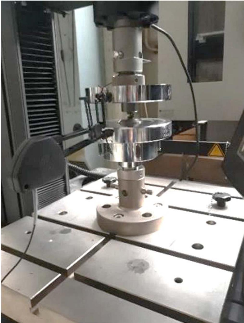
**Figure 7:** Setup for testing the compression behavior of the c-rings.
