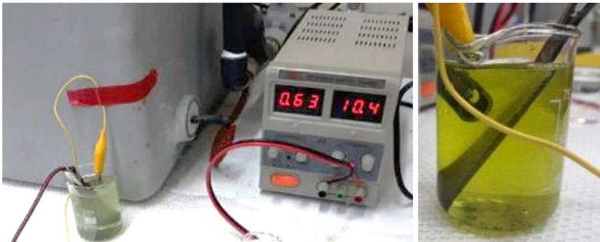
**Figure 29:** Electrochemical cleaning of NiTiHf specimen.
