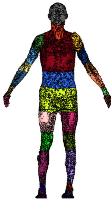
Figure 7. IAVCA body re-segmentation. To reposition a model into different poses, we re-segmented it into 53 new parts.
