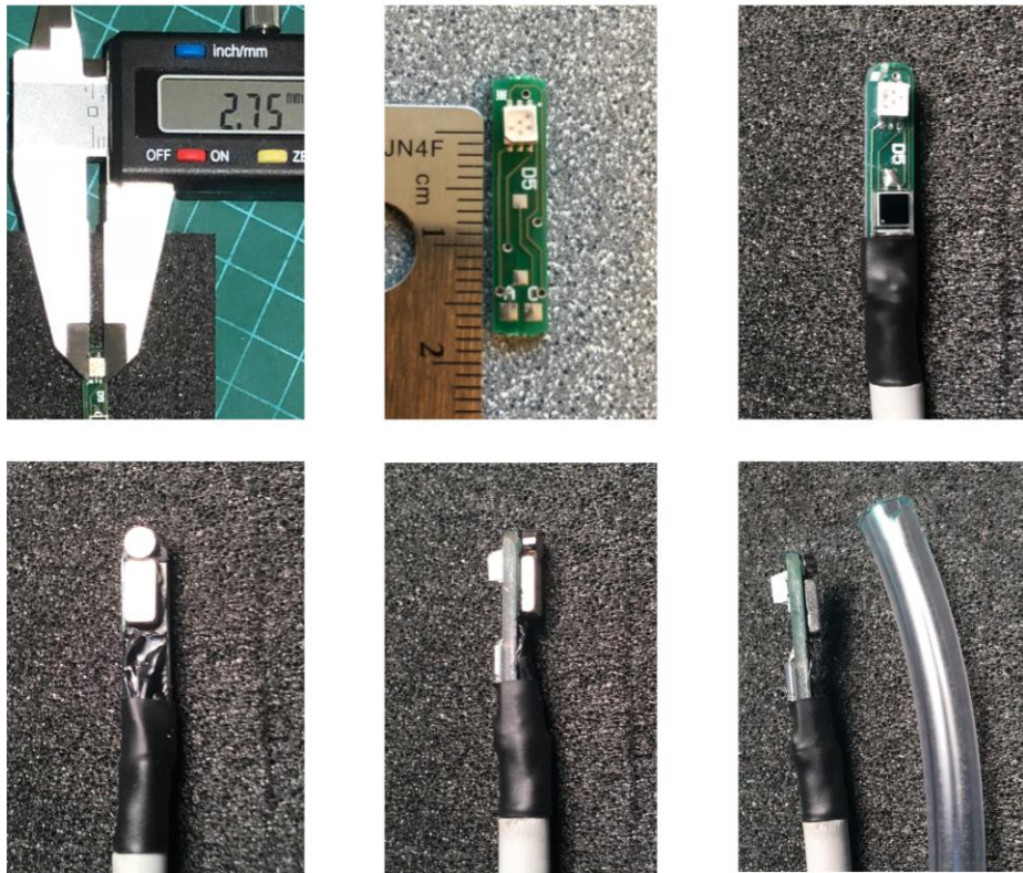
Figure 2. V2 SC-NIRS sensor prototype model - optode components and structure.
