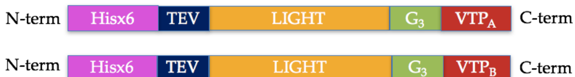
Figure 1: Visual representation of LIGHT-VTP protein sequence. DNA sequences from left to right include: 6x histidine tag, tobacco etch protease site, LIGHT, 3x glycine linker, and vascular targeting peptide.
