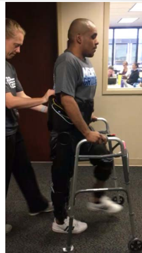
Study 2 subject walking with FES-assisted exoskeleton.
