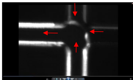
Figure 12. Screen capture of video showing flow in microfluidic device. Water is being driven by positive pressure from syringe pumps from top, bottom, and right channels. Waste is going to channel on left after four-way junction.
