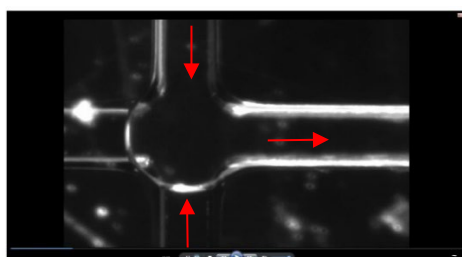
Figure 14. Screen capture of video showing flow in microfluidic device. Water is being driven by positive pressure from syringe pumps from top and bottom channels. Negative pressure is acting on the waste channel to the right, pulling the liquid.
