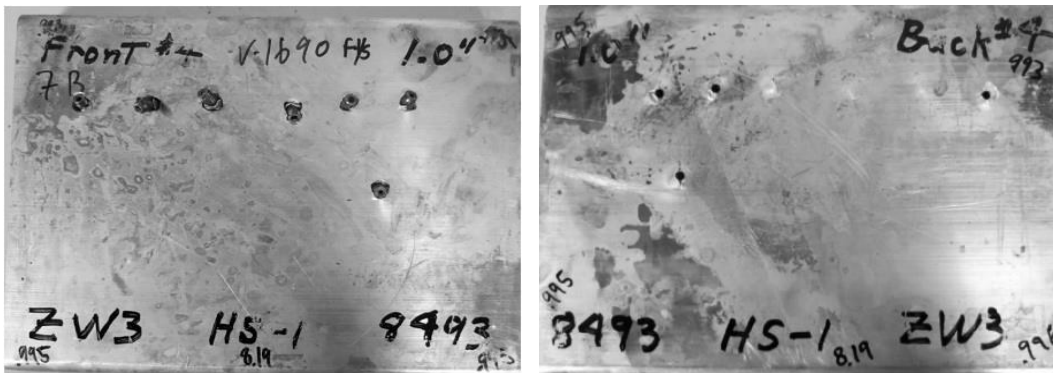
Fig. 16 ZK60A-T5 25-mm profile target vs. 0.30-cal. APM2, 0° obliquity, front (left) and back (right)
