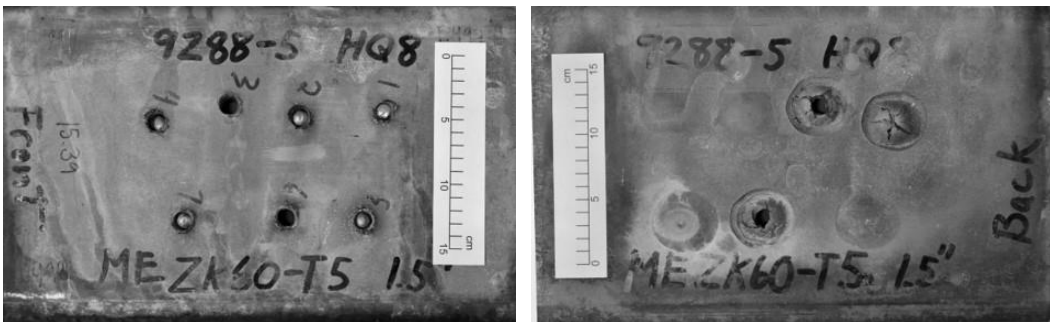
Fig. 20 ZK60A-T5 38.1-mm profile target vs. 0.50-cal. FSP, 0° obliquity, front (left) and back (right)
