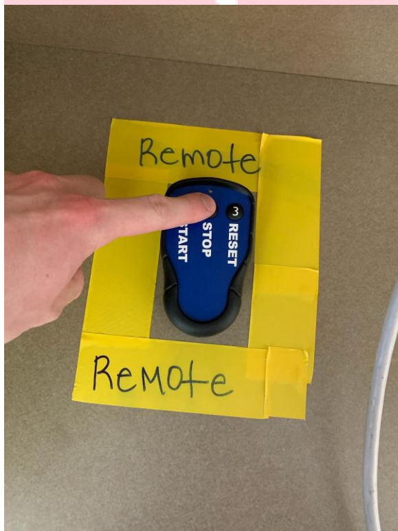
Figure 15 – Stop cycle on remote as soon as possible after minimum required dose.
