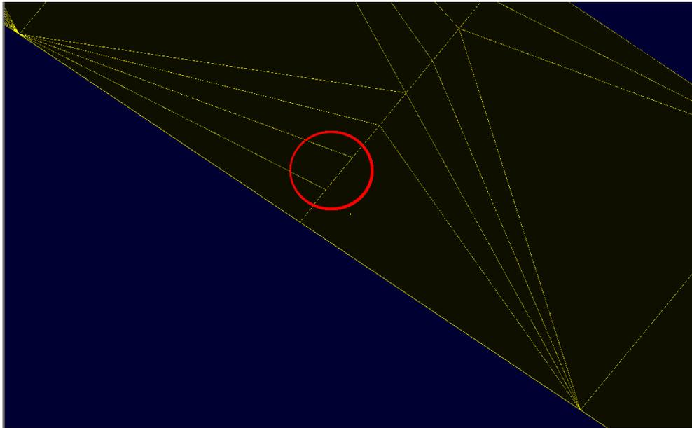
**Figure 12. Example of incorrect triangulation due to linearity of sampled points**
