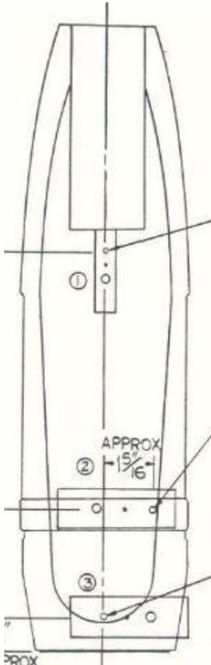
Figure (1) Drawing of IQI placement for an M1 shell [4]
