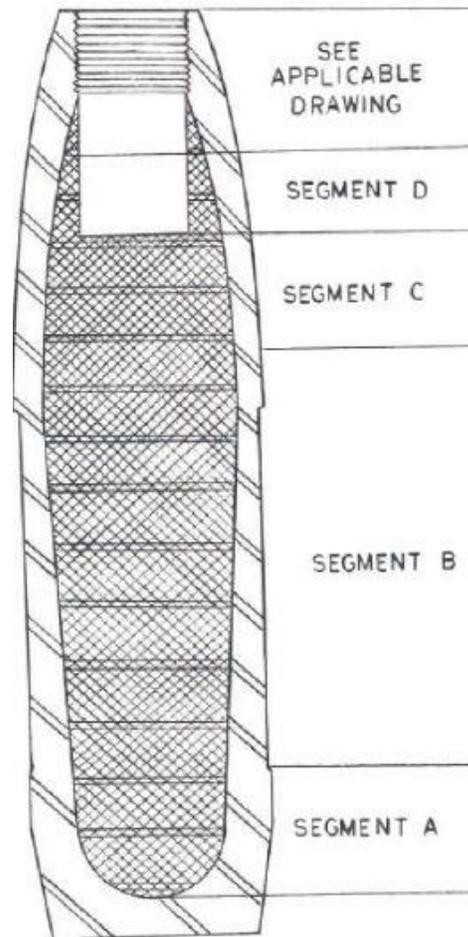
Figure (4). Segments of an M1 Shell. [4]
