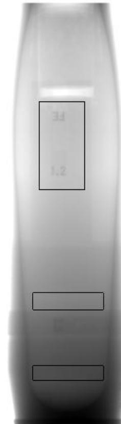
Figure (2) Depicted is a radiograph of an M1 shell. The rectangular regions are the regions of interest submatrices near the IQI placement
