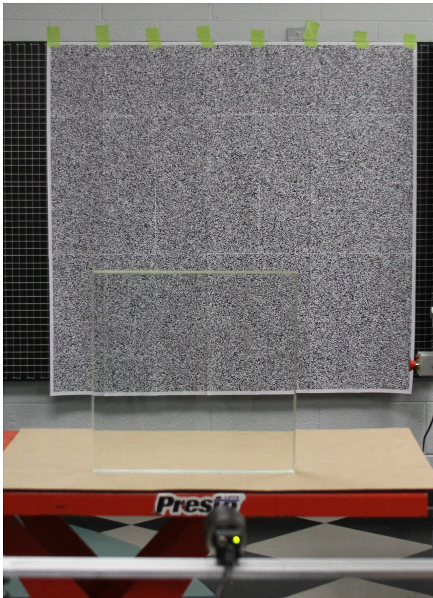
Figure 1: The experimental setup used to measure the distortion of the TA. As the reader can see, the only real difference in the setup between the standards [2, 3, 4] and the present case is the use of a printed speckle pattern instead of the grid lines.
