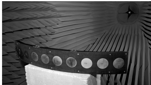
Figure 9.9 3D-printed non-planar array under test.
