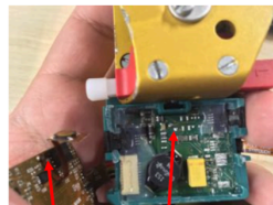
Remove Switch Solder to Our Board
