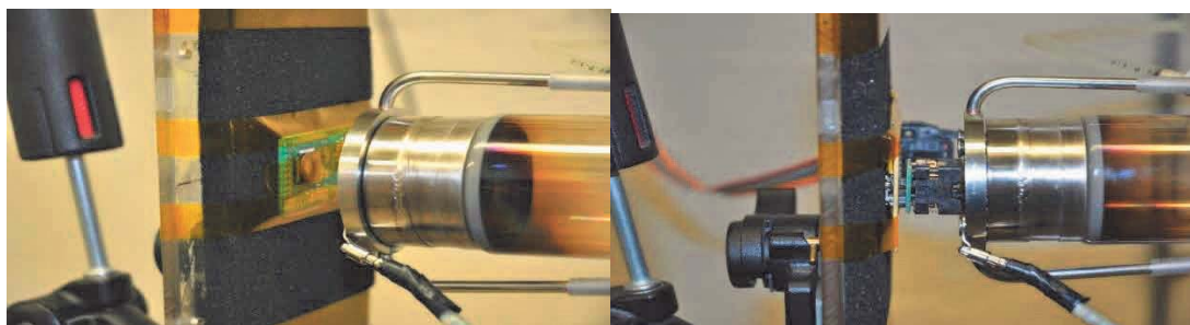
Figure 7. The in-situ testing setup of neutron radiation for Panasonic chip and Adesto chip
