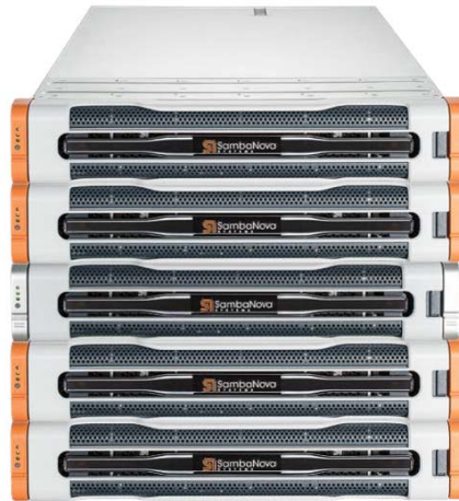
Figure 8: SambaNova SN10-8 System with 12 TB DRAM in \frac{1}{4} Rack
