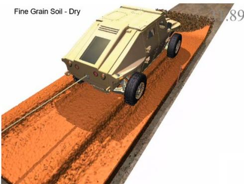
**Figure 1** Snapshot from a DIS drawbar-pull simulation for a wheeled vehicle on a dry fine grained soil.
