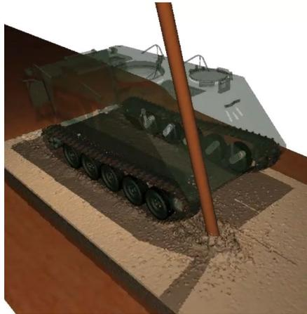
**Figure 30** DIS simulation of tracked vehicle overriding a pole embedded in the DEM soil.
