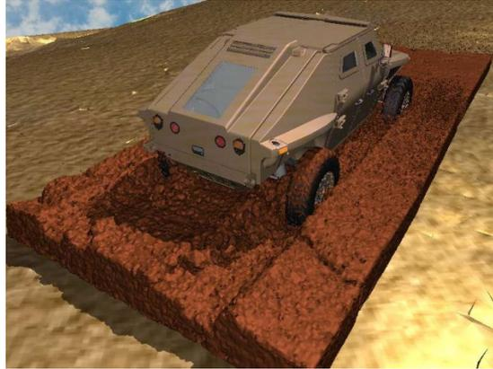
**Figure 20** DIS simulation of a vehicle going over a soft soil terrain which includes adhesion between the tires and the soil.
