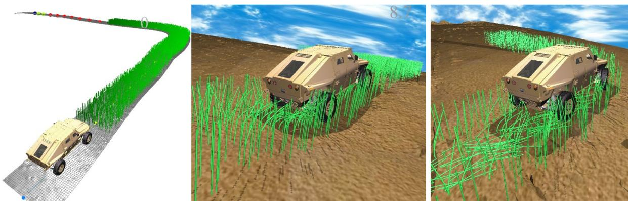
**Figure 28** DIS simulation of a wheeled vehicle over a crop/grass covered terrain. The right figure shows the breaking of the breaking of the vegetation blades behind the vehicle.
