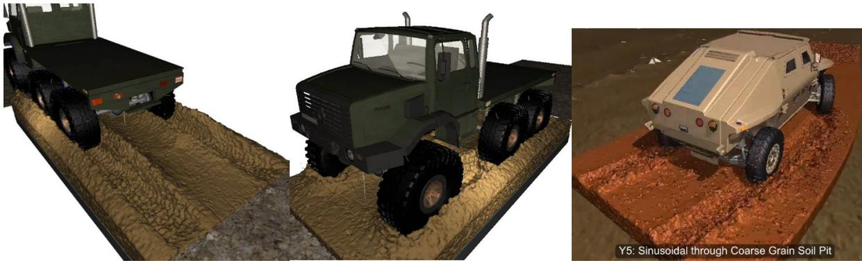
**Figure 5** DIS simulations of wheeled vehicle on soft cohesive soil showing deep side ruts (left), soil bulldozing in front of the tires (center), and soil separation/reattachment during sinusoidal steering (right).
