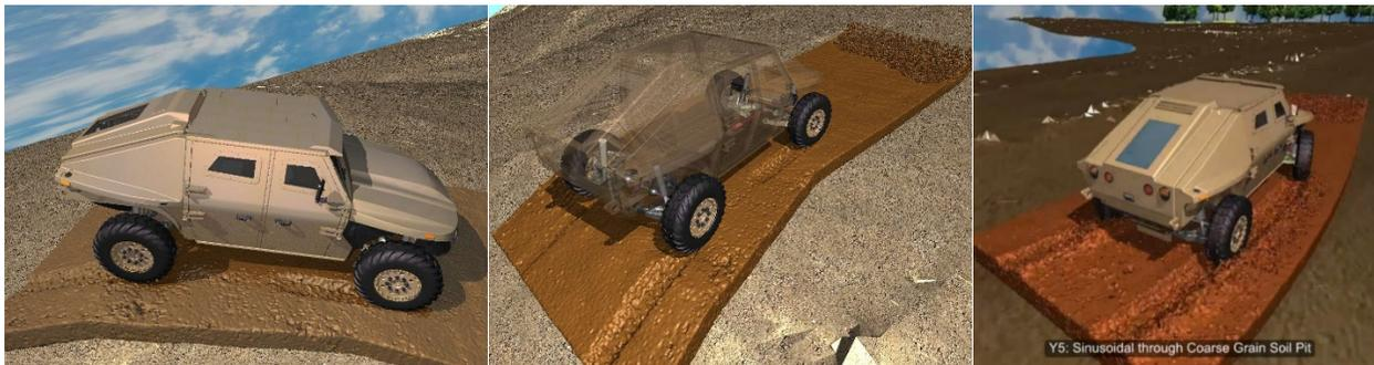
**Figure 27** Coupled DIS MBD/DEM simulation of a wheeled vehicle using a complex topography moving soil patch and about 1M particles which includes up/down slopes, turns, and surface roughness.
