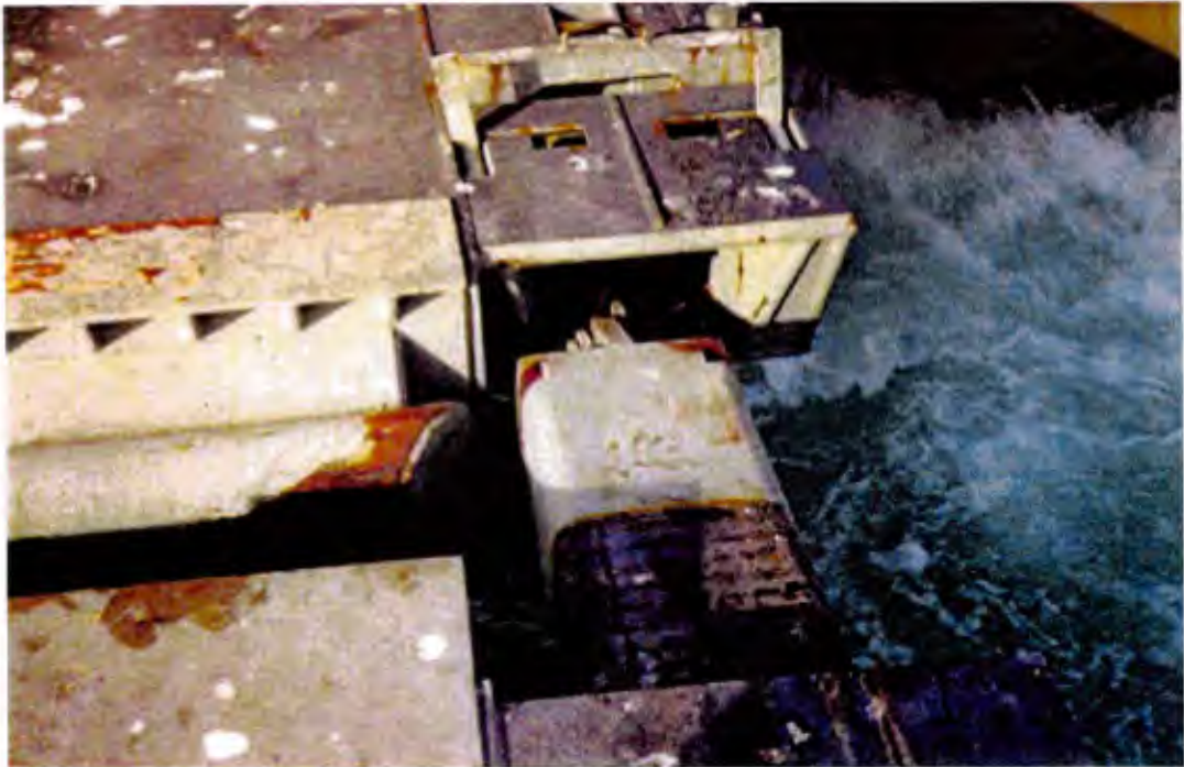
Figure 15 Misalignment of Flexor head and receiver opening causes momentary binding.
