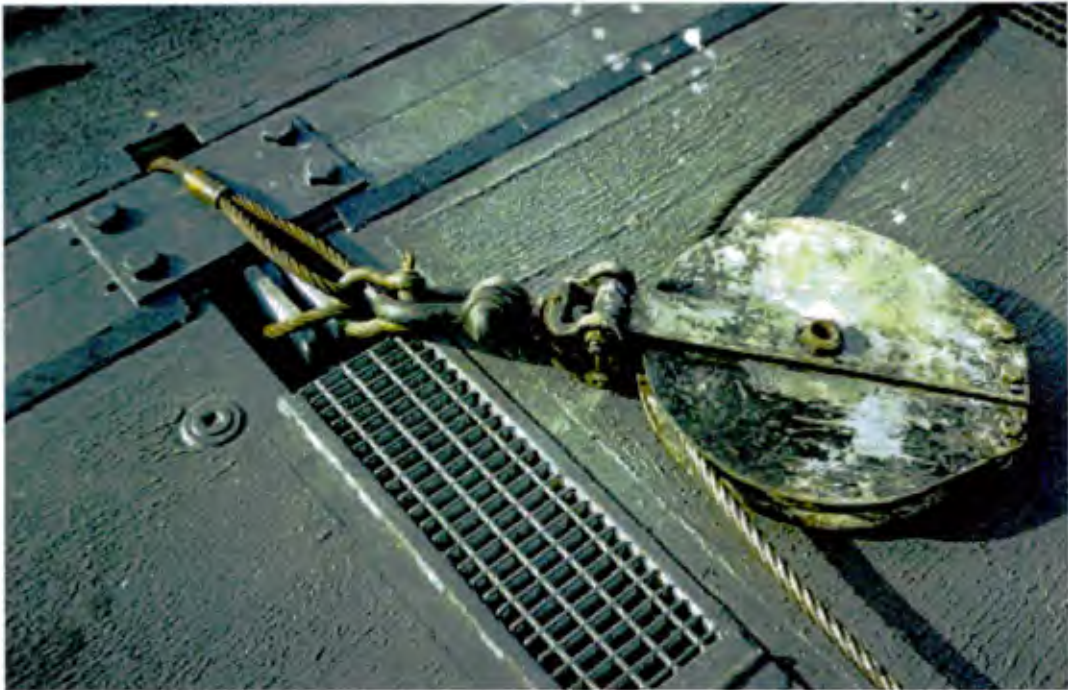
Figure 10 Wire strap around angle and PH-6 padeye rigged to place 18-inch snatch block on the centerline of the causeway.
