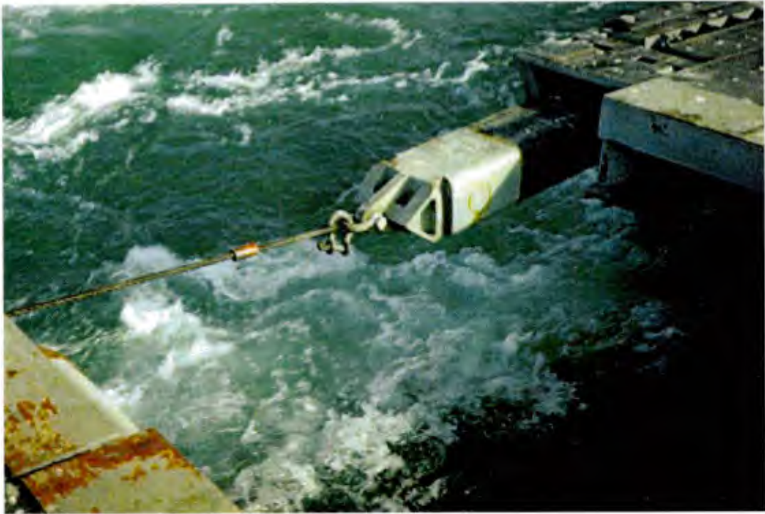
Figure 14 Upset anchor shackles poses a potential jamming problem.
