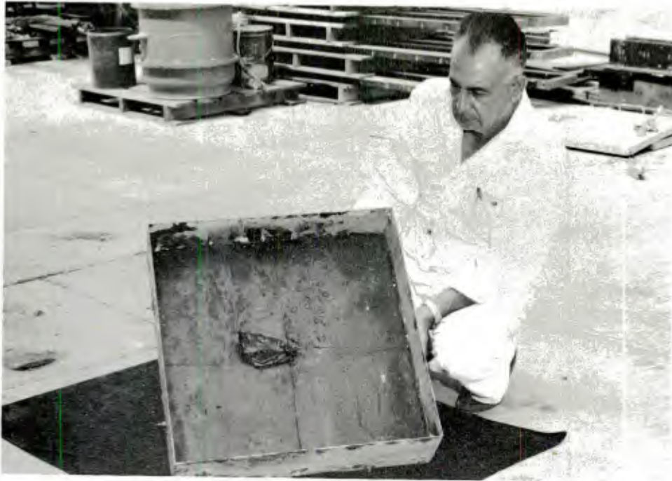
Figure 12. Interior view of Figure 11 showing plastic bag which contained copper sulfate crystals.
