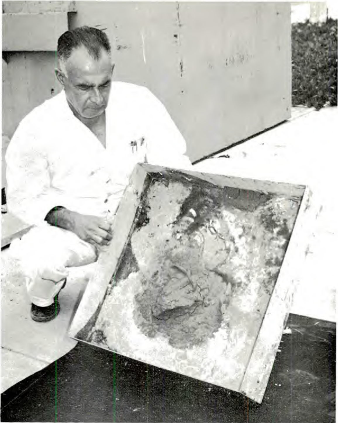
Figure 9. Interior view of recovered concrete footing with aluminum skirt.
