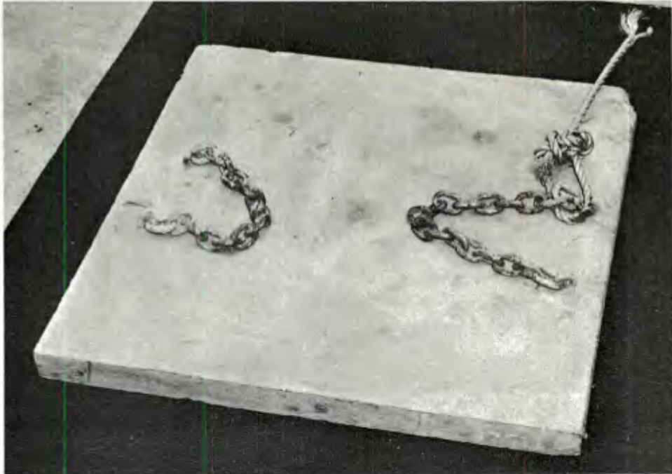
Figure 6. Recovered 2-foot square concrete footing.
