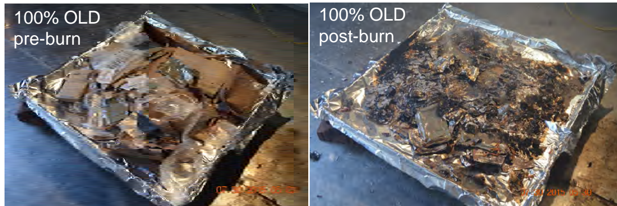
Figure 37. MRE (100 % OLD material or 0 % NEW) on 3.2 x 3.2 foot steel pan, before (left) and after (right) burn.
