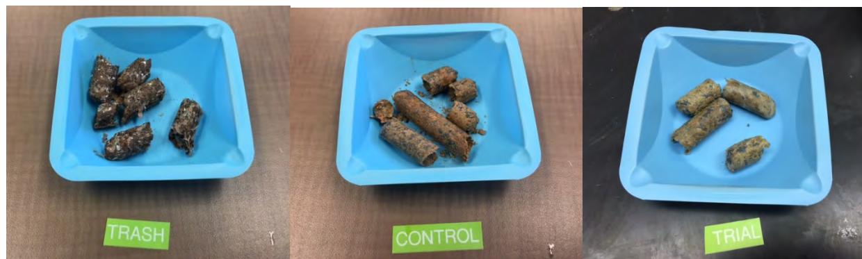
Figure 95. Pellets after filtering out the fines, from left to right, made from 12/5/16 trash, Recipe #2 control feedstock, Recipe #2 trial feedstock
