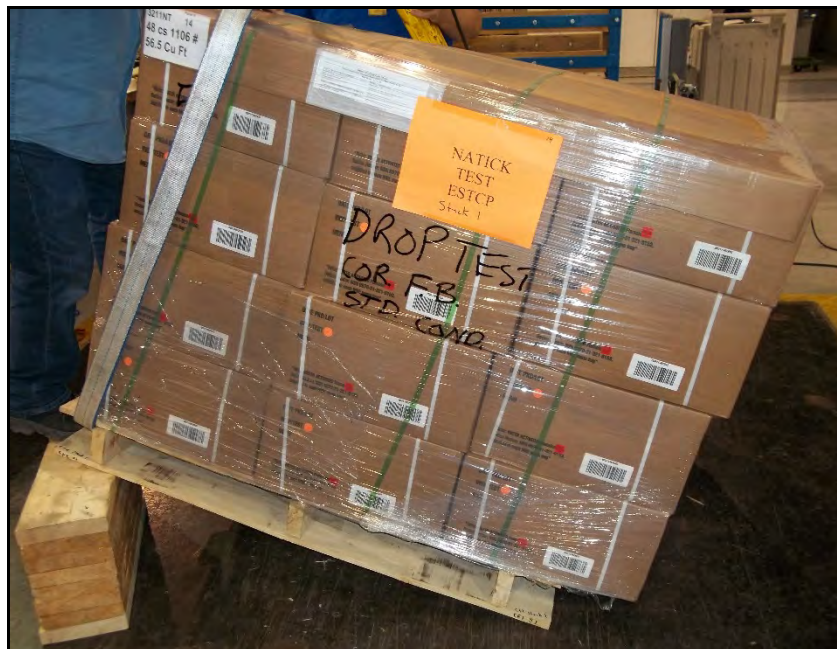
Figure 14. Rotational Corner Drop
