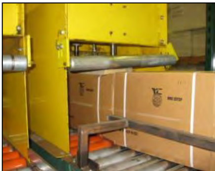
Figure 63. Deflection of containers caused by the pressure of the container staggering system
