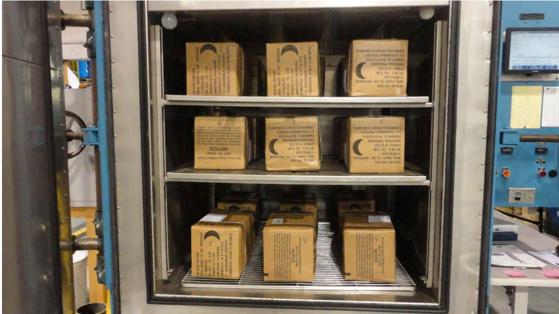
Figure 18. MREs in Altitude Chamber
