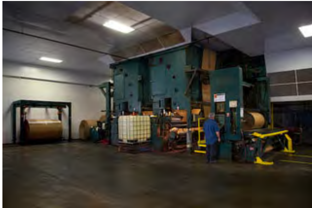
Figure 43. Coating paper with the Spectra-Kote
