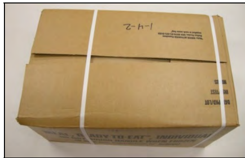
Figure 113. Excessive gap width of \frac{3}{4} inch or greater between the major flaps, normally caused by over-packing
