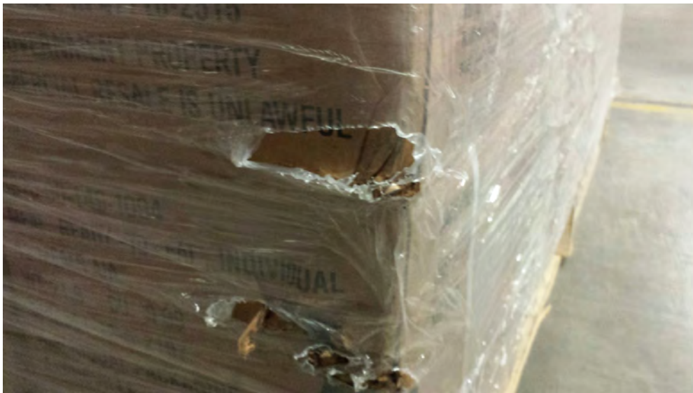
Figure 93. Significantly damaged edge of a pallet.
