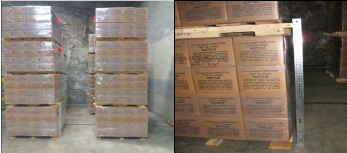
Figure 67. Stacks of MRE cases at Marengo Caves (left) and the deflection measurement system (right)
