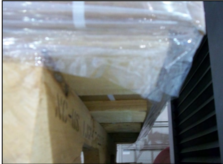
Figure 78. Solid Fiberboard Case Deformation (High Humidity Conditions)
