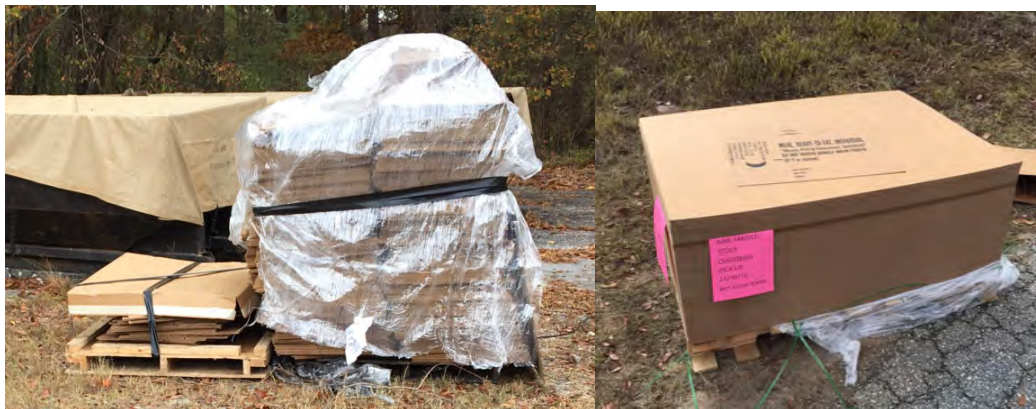
Figure 34: Trial corrugated cardboard/fiberboard on left, control fiberboard on right
