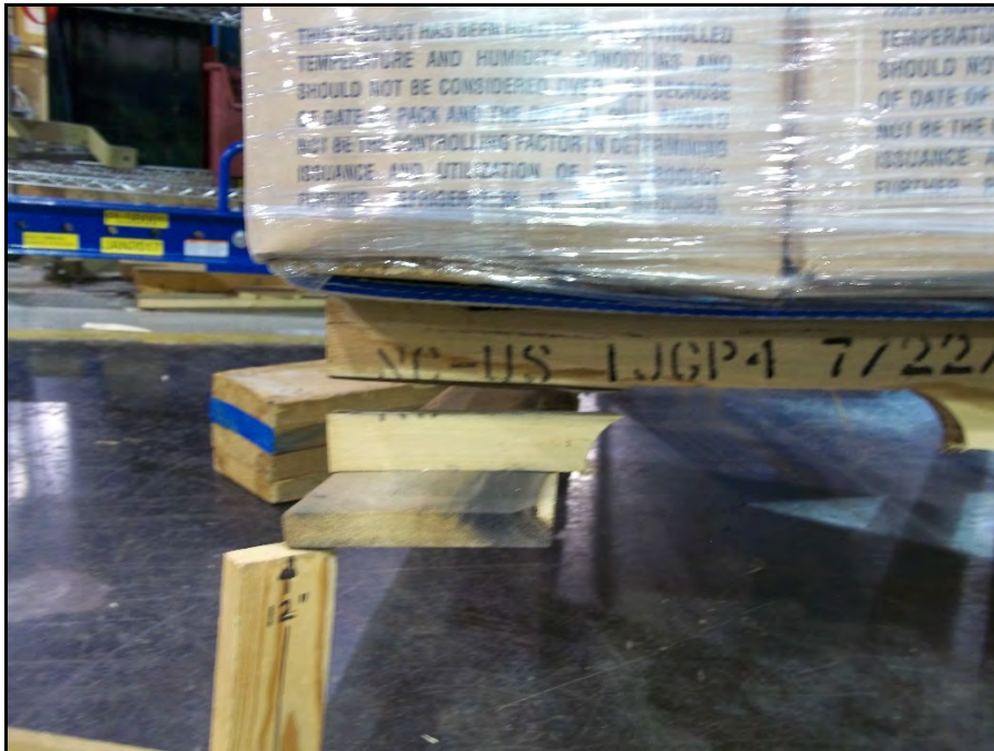
Figure 83. Cracked Stringer During Rotational Drop Tests
