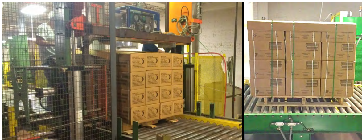
Figure 59. Images of the unitization of current MRE rations (48 cases per load) (left) and a fully-strapped unitized load (right)
