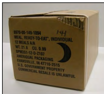
Figure 117. Superficial damage to container during material handling operations or damage from case assembly equipment
