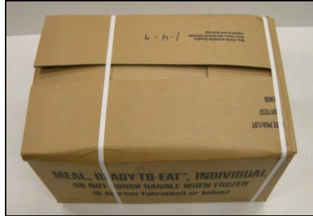
Figure 115. Misaligned straps due to the larger case size, issue can be corrected through adjustment of strapping systems
