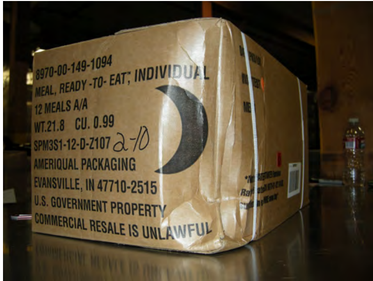
Figure 128. Dents on Pallet #1 Layer 2 Box 10
