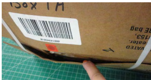
Figure 76. Glue separation on Solid Fiberboard
