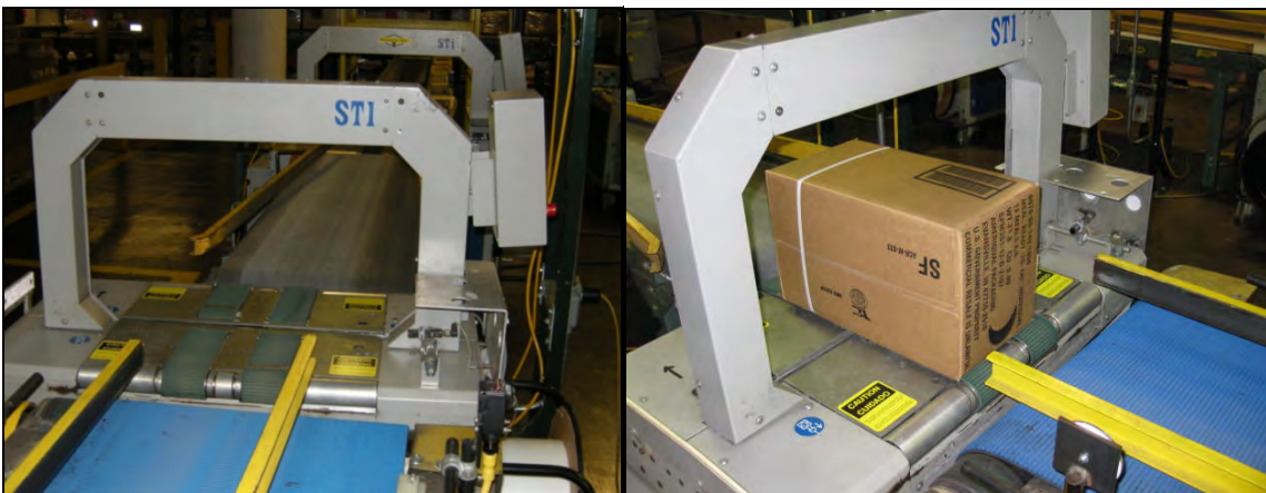
Figure 56. Case Strapping equipment used to band individual containers (left) and the strapped case (right)
