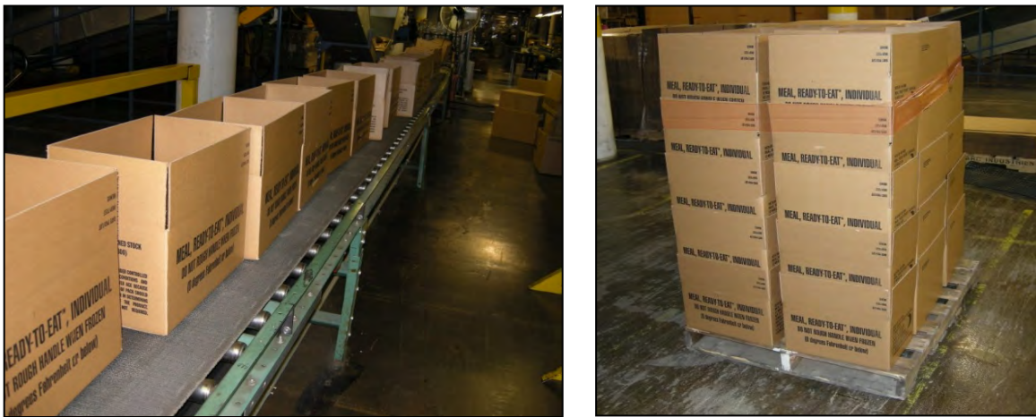
Figure 46. Corrugated test samples manufactured by York Containers on the AmeriQual MRE assembly line (left) and erected on a pallet (right)
