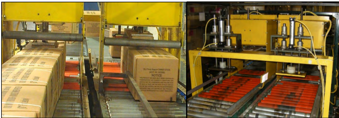
Figure 57. Case mixing equipment developed by AmeriQual Packaging (left) and a view of the front gate (right)
