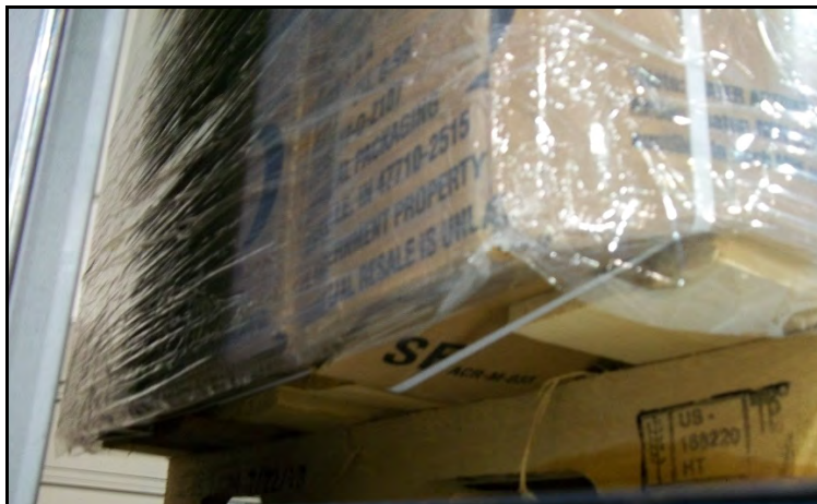
Figure 77. Corrugated Fiberboard Case Deformation (High Humidity Conditions)
