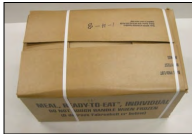
Figure 119. False scores on major flap caused by over-packing of container
