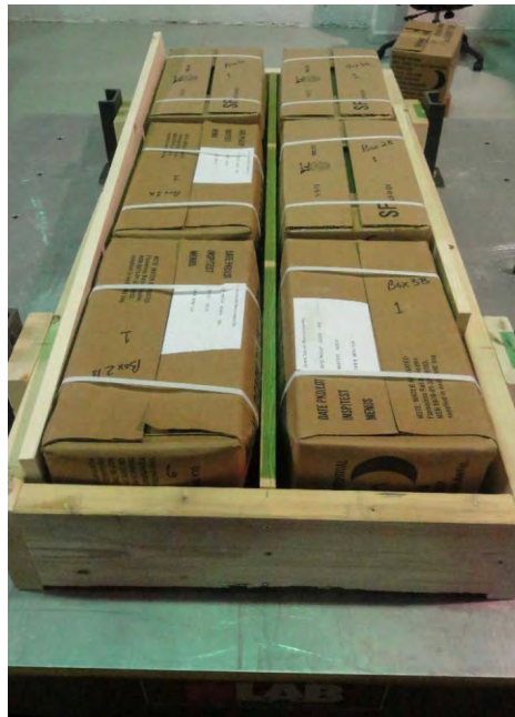
Figure 23. MREs during Random Vibration
