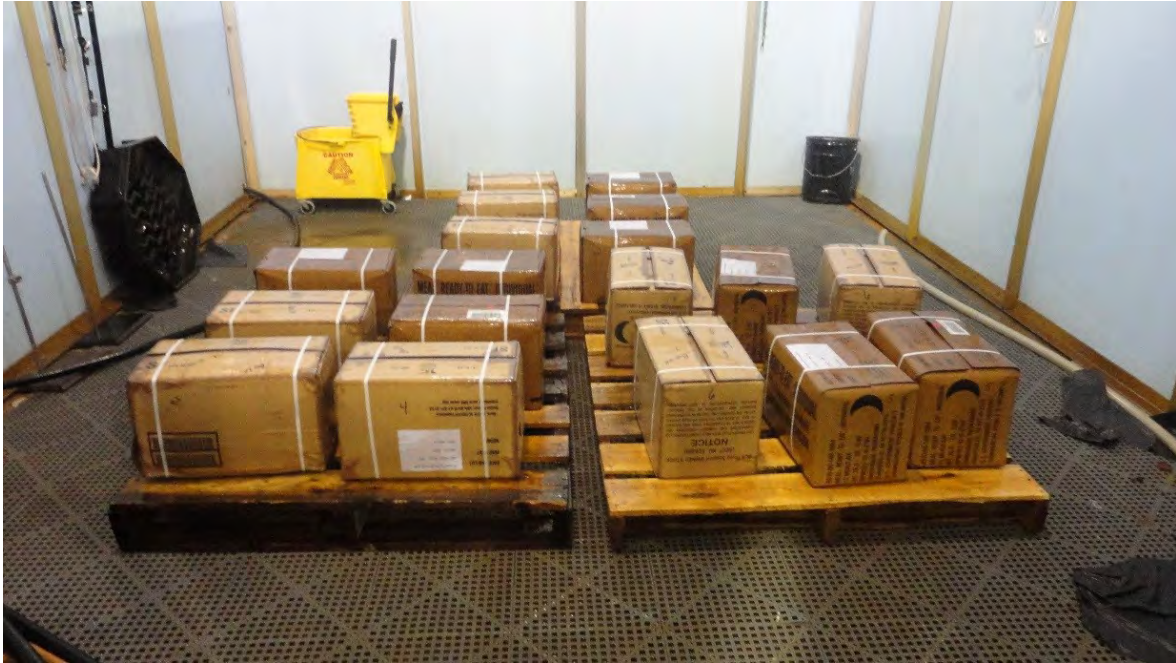
Figure 19. MREs Under Rain Test
