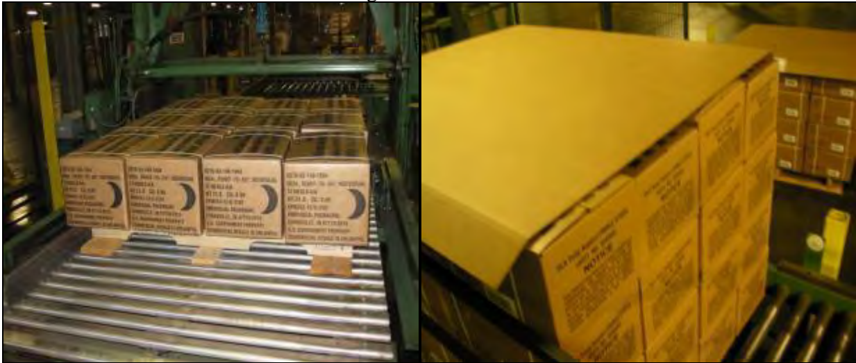
Figure 64. First level of containers in the palletizer (left) and the problem identified with the location of the cap folds on pallets of new containers (right)
