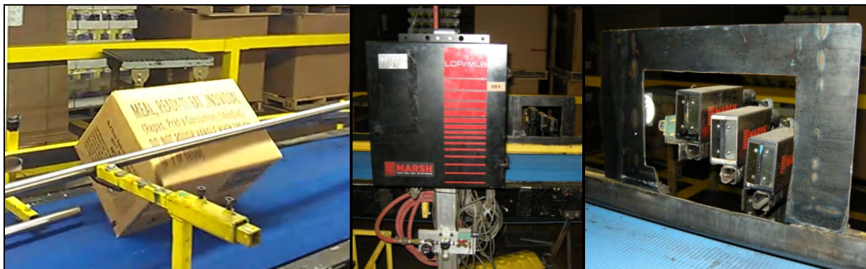
Figure 54: Orientation of container prior to print (left), Marsh LCP/ML8 printing station (middle) and three print heads (right) used to print the date of pack, inspection test date and case identification
