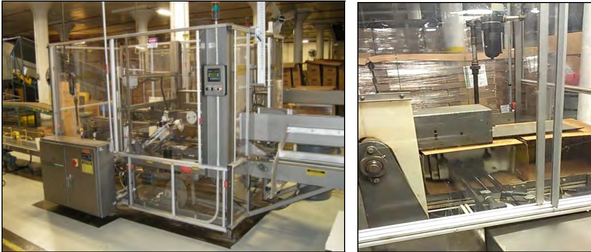
Figure 47. Full view of the case erecting equipment from Pearson Packaging Systems (left) and close up of the gluing of the container's bottom flaps (right)
