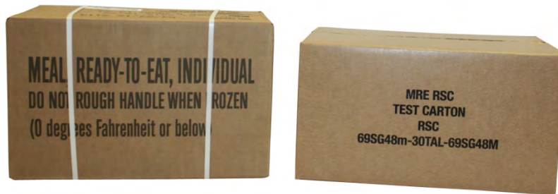
Figure 1. MRE containers, current solid fiberboard (on left) and prototype corrugated container (on right).
