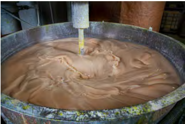
Figure 41. Blending the coating formulation
