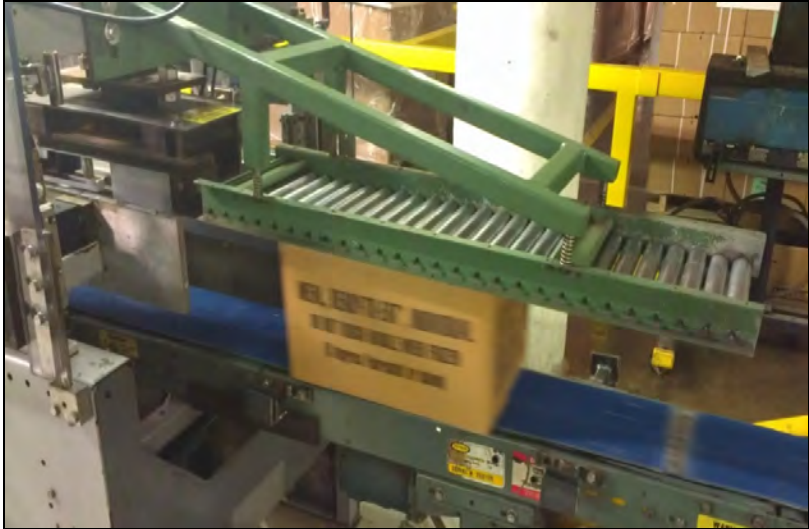
Figure 52. Conveyor system used for securing glued flaps during curing of adhesive
