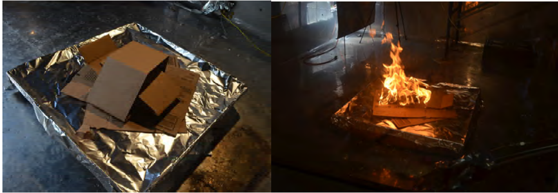
Figure 36. The paperboard test material (corrugated Spectra-Kote Polymer Fiberboard box and liner) atop aluminum foil (left) on 1 m x 1 m (3.2 ft x 3.2 ft.) steel pan. Combustion of same (right).
