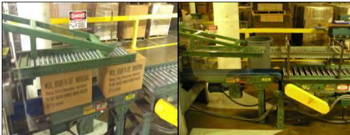
Figure 62. Case sealer prior to (left) and after (right) the closure seal modification
