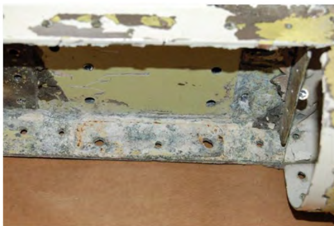
Figure 97: Photograph illustrating T-45 Rudder lower fitting attachment area with significant spar corrosion in the fitting attachment areas.
