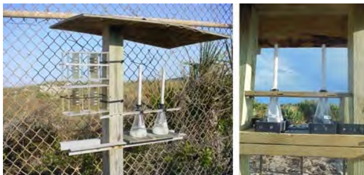
Figure 18: Wet Candle Exposure Fixtures at Whidbey NAS (left) and Canaveral AFS (right)
