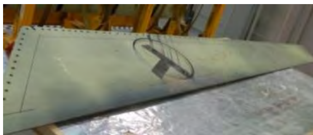
Figure 99: Damaged area on F/A-18 leading edge of vertical stabilator.
