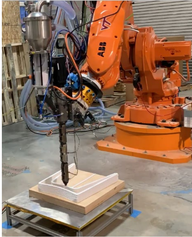
Figure 18 Virginia Tech Large-Scale Robotic Extrusion System, which features a ~8 foot reach and 150 lb/hr pellet extrusion
