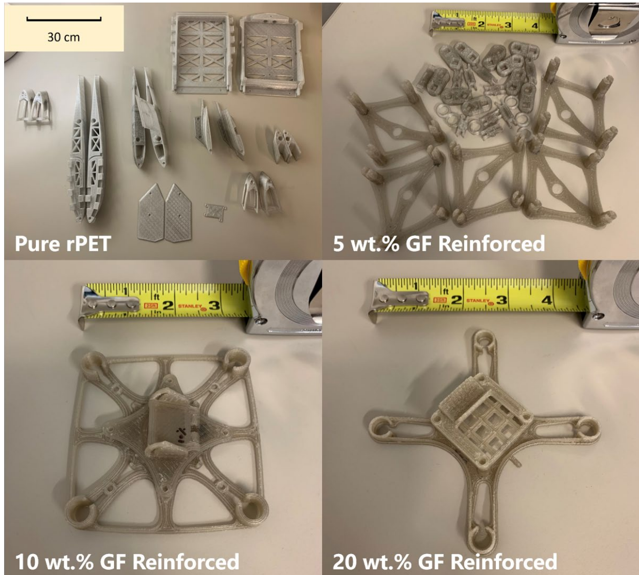
Figure 7 Various complex parts of autonomous aerial vehicles printed with rPET/GF filaments
