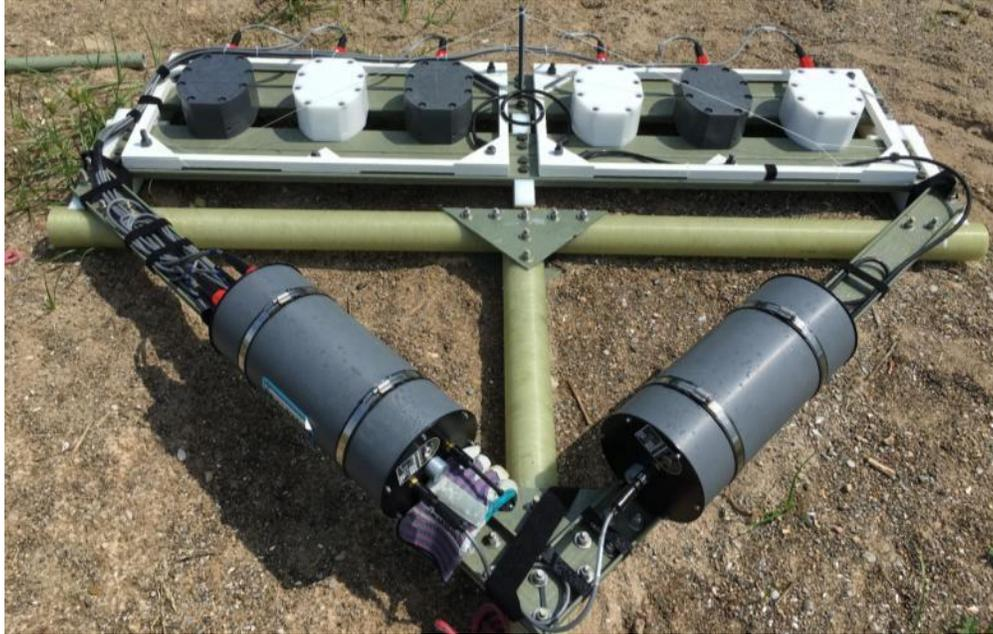
**Figure 6. Photograph of the FlexEM array including the transmitter (foreground, right side) and receiver (foreground, left side) electronics pressure vessels, the sled attachment, and transmitter and receiver components mounted to the FRP sled system.**
