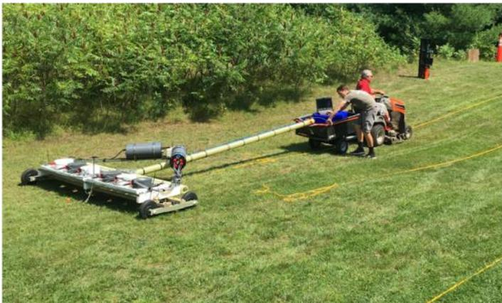
**For dynamic survey tests, the system was mounted on a set of wheels and towed from a lawn tractor.**
