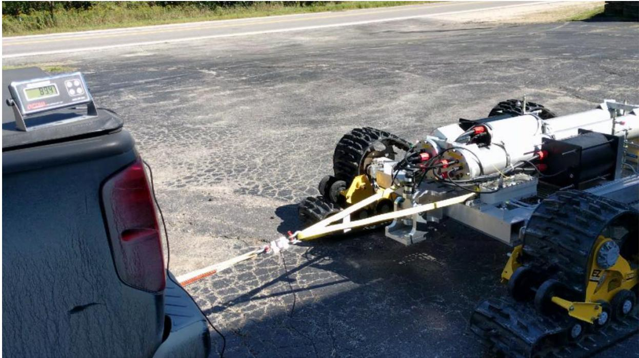
**Figure 17. Photographs of the bollard pull force test set up and configuration.**
