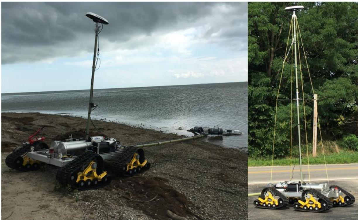
**Figure 11. Photograph of the crawler system with dual heading RTK DGPS rover attached to its mast (Left). The extended GPS mast and tensioned stays are shown with antenna 6.5 meters above the ground (Right).**
