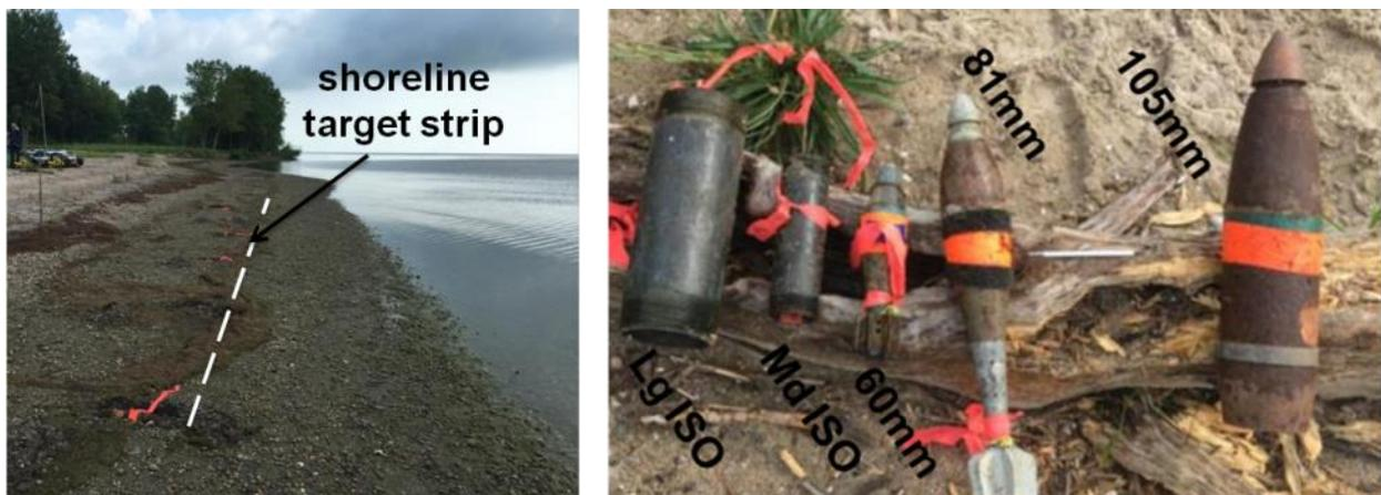
Figure 33. The shakedown test area including target strip at the initial water line (the water line shifted or receding during our tests). The locations of the 5 targets we used are shown in the photograph parallel to the shoreline.
