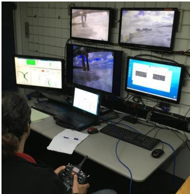
**Figure 27. The topside operator control station with multiple operator displays. These include (from left to right) the navigation and mission control user interface, 3 crawler-based cameras, the FlexEM array data acquisition and real-time display, the power management system interface and scanning sonar display.**
