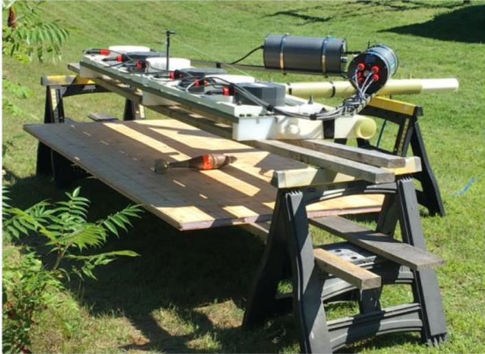
**Figure 25. Photographs of the experimental test stand and dynamic test area for dry characterization tests. A select set of targets were used to characterize the array performance in both the test stand and buried in the test field.**
