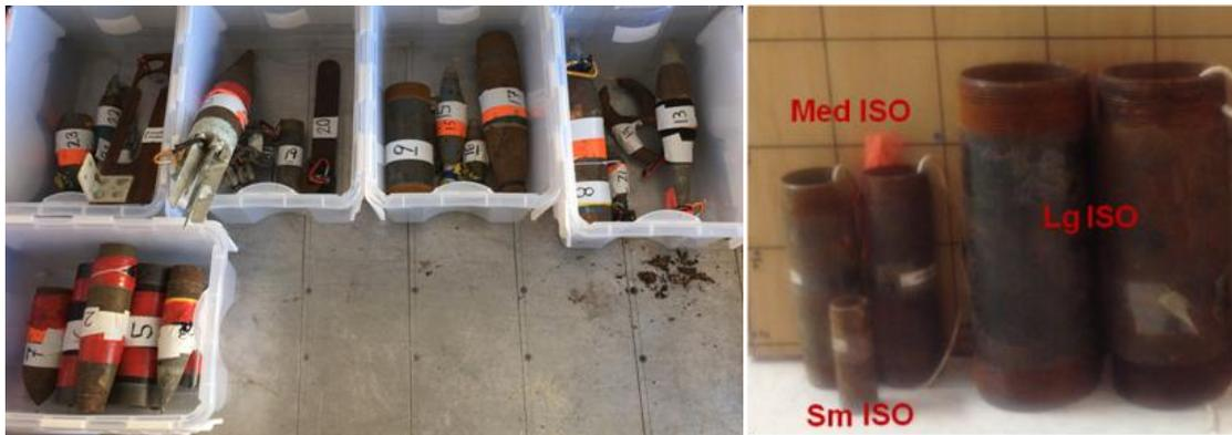
Figure 59. Photographs of the simulant targets used in the demonstration. These include ISO's, simulant UXO from the Aberdeen Test Center (ATC) test set, clutter objects, and other canonical metal objects for assessing the performance of the overall system.
