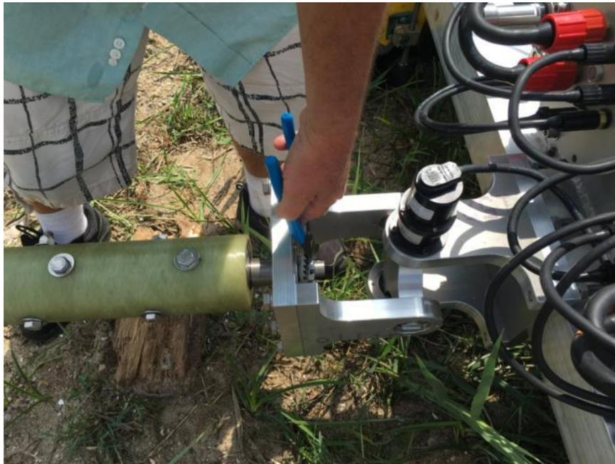
**Figure 9. Photograph of the 3 DOF tow point hitch and incremental angle encoder on the aft portion of the crawler. The marine-grade encoder supplies serial data to the multiplexer and fiber optic tether modem for topside data logging and integration with other navigation and positioning information.**
