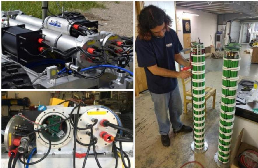
**Figure 2. Photographs of the cylindrical battery pod pressure vessels and battery cell stacks. Each stack contains 600 Li-ion cells to produce a total of 7.5 kWh power supply.**
