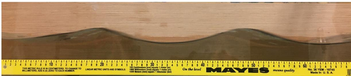
Figure 6. Design of a small wave tank using a flap paddle driven by a rail mounted stepper motor to generate waves of specific wavelength and amplitude. An absorbing beach is placed at the back of the test tank to prevent wave reflections. A sample of actually waves generated in the tank with a measured wavelength of  $\sim 29$  cm. The target wavelength for this test was 29.5 cm.
