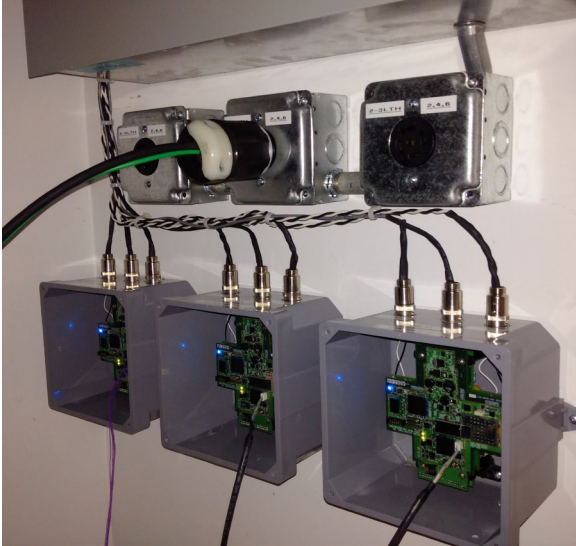
Figure 2-5. Echo Hardware in Three-phase Box Form Factor (using CTs for Current Measurement)
