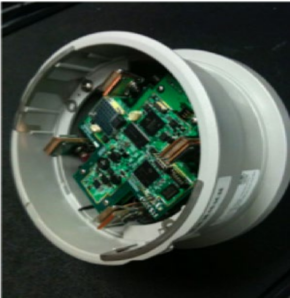
Figure 2-4. Prototype Residential Echo Module Designed to Fit in the Kilowatt-hour Meter’s Form Factor
