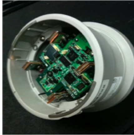
Figure ES-3. The Prototype Residential Echo Module, Designed to Fit Under the Electric Service Meter
