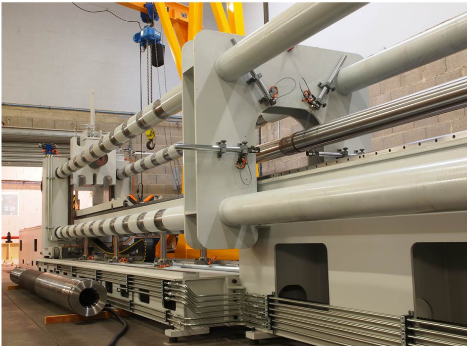
Figure 5: Horizontal High Pressure processor (Top: NC Hyperbaric; bottom: Thiot)
