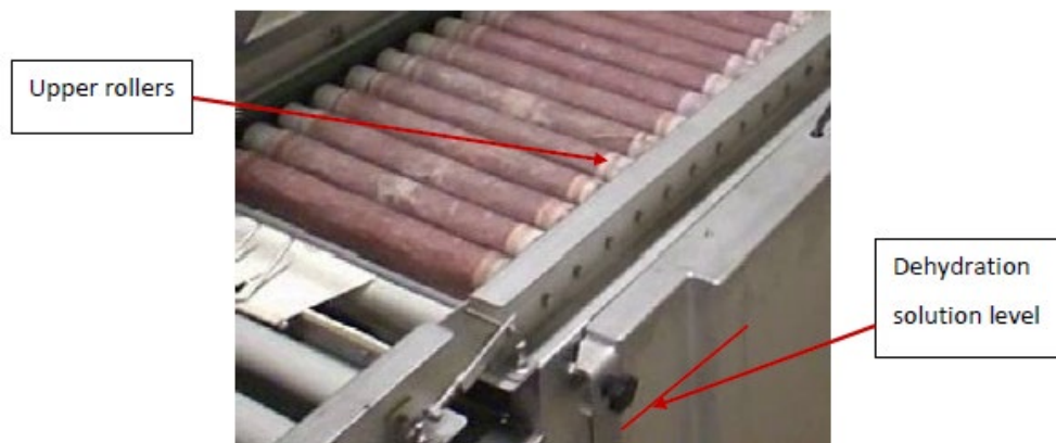
Figure 2: Rollers to guide the conveyor into the Osmo tank
