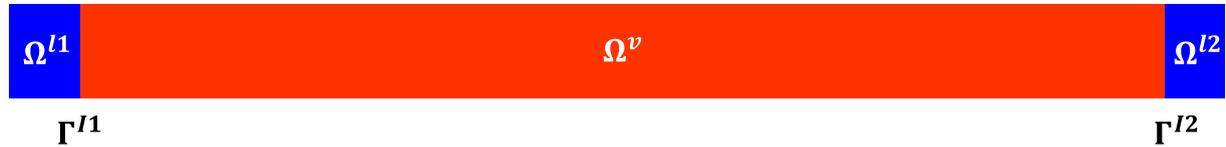
**Fig. 1.** 2D schematic of the considered problem.  $\Omega^{l1}$  and  $\Omega^{l2}$  are the two liquid (blue) regions,  $\Omega^v$  is the vapor (red) region.  $\Gamma^{l1}$  (evaporation) and  $\Gamma^{l2}$  (condensation) are the liquid-vapor interfaces. (For interpretation of the references to color in this figure legend, the reader is referred to the web version of this article.)
