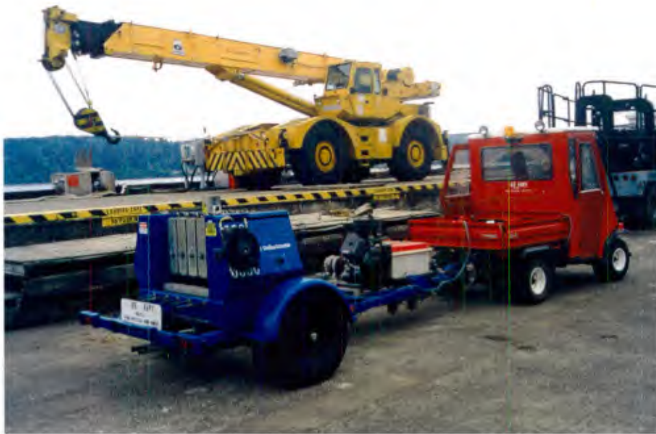
Figure 10. Falling weight deflector and tow vehicle on Marginal Wharf.
