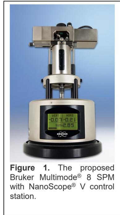
**Figure 1.** The proposed Bruker Multimode<sup>®</sup> 8 SPM with NanoScope<sup>®</sup> V control station.
