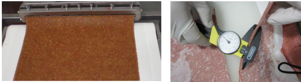
Figure 7: Actual extrusion of meat (left); measurement of meat thickness (right)
