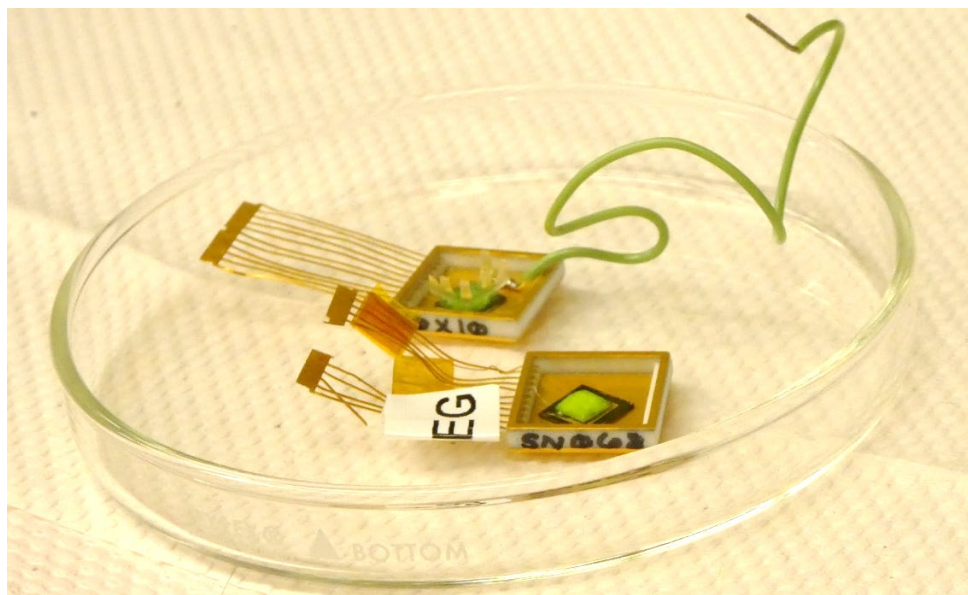
Fig. 1 Fully packaged Widetronix Inc. planar and textured SiC devices loaded with ^{63}\text{NiCl}_2 (green)
