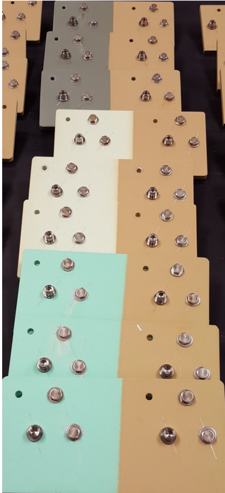
Fig. 6 MIL-DTL-81706 Type II: top three primed with MIL-PRF-23377 Class C, middle three primed with MIL-PRF-23377 Class N, and bottom three primed with MIL-PRF-85582
