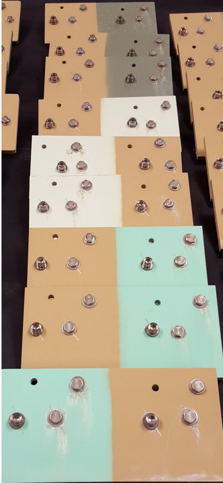
Fig. 10 3M AC131: top three primed with MIL-PRF-23377 Class C, middle three primed with MIL-PRF-23377 Class N, and bottom three primed with MIL-PRF-85582
