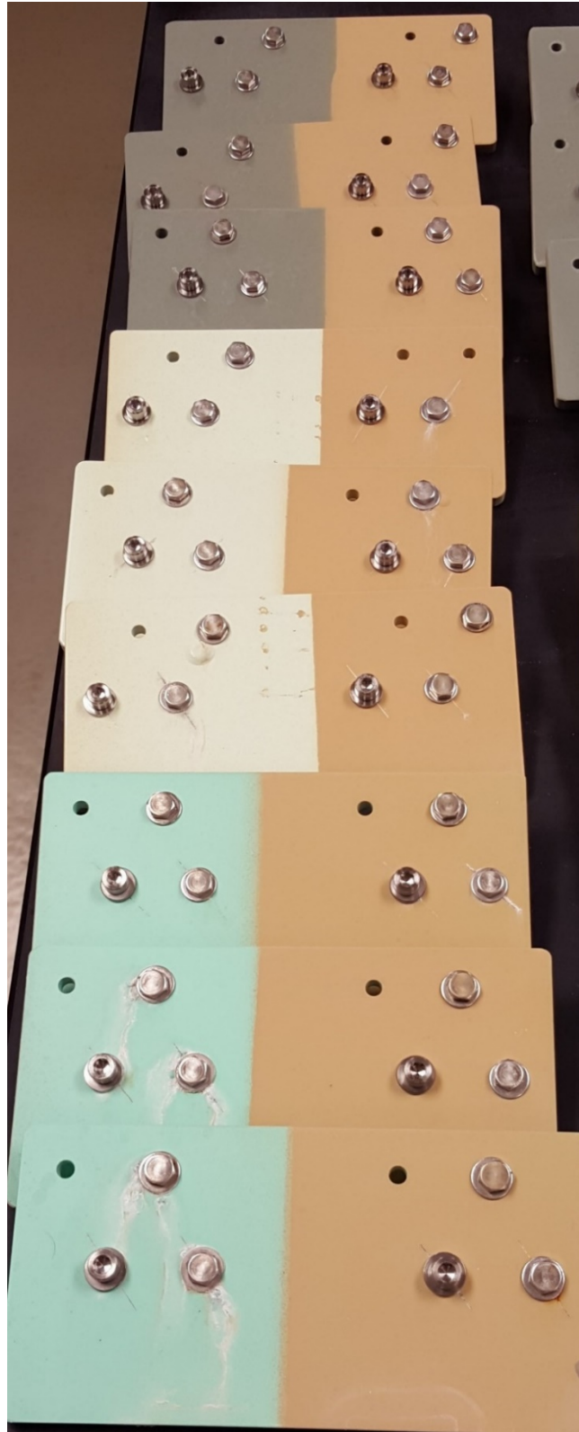
Fig. 5 MIL-DTL-81706 Type I: top three primed with MIL-PRF-23377 Class C, middle three primed with MIL-PRF-23377 Class N, and bottom three primed with MIL-PRF-85582
