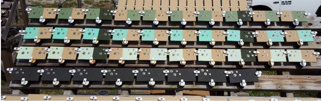
Fig. 4 Racks at CCAFS/TACOM outdoor exposure site with galvanic panels on the top three rows
