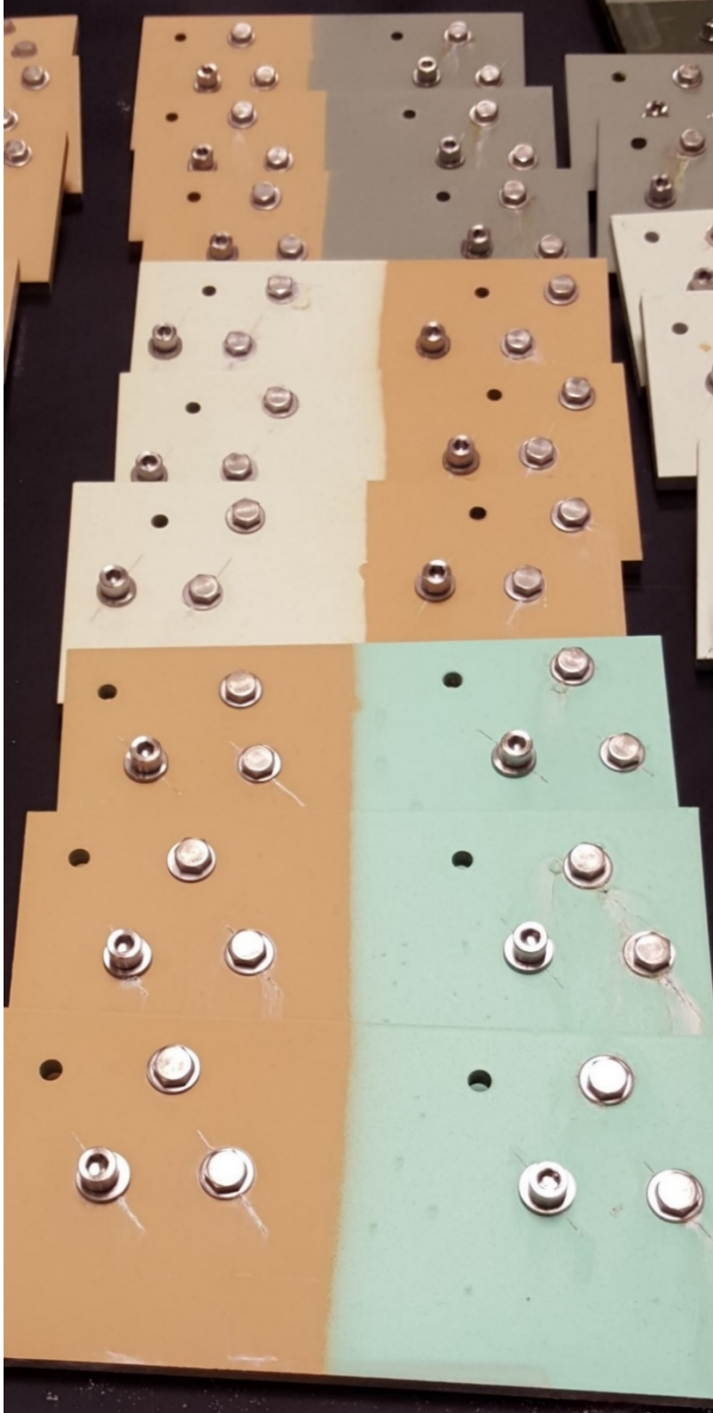
Fig. 7 Henkel 5700: top three primed with MIL-PRF-23377 Class C, middle three primed with MIL-PRF-23377 Class N, and bottom three primed with MIL-PRF-85582
