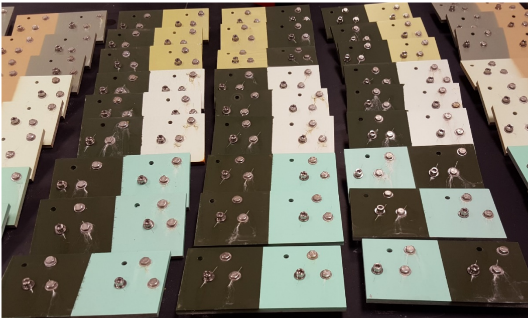
Fig. 11 Deft 1043(L), DFS (C), and 1060(R): top three primed with MIL-PRF-23377 Class C, middle three primed with MIL-PRF-23377 Class N, and bottom three primed with MIL-PRF-85582
