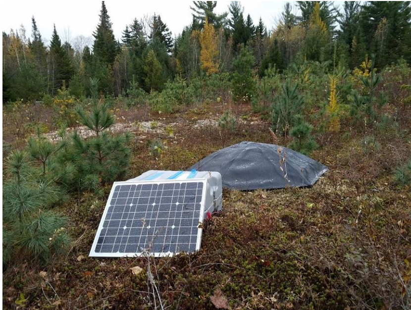
Figure 7. Station WARR equipped with L-4 seismometer and an acoustic sensor (Hyperion IFS-5311). The acoustic sensor is covered with a wind noise-reducing dome.
