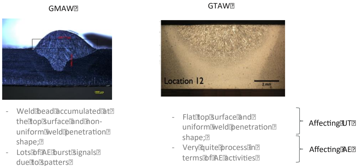
Figure 6 Difference in weld morphologies and process noise for GMAW and GTAW.
