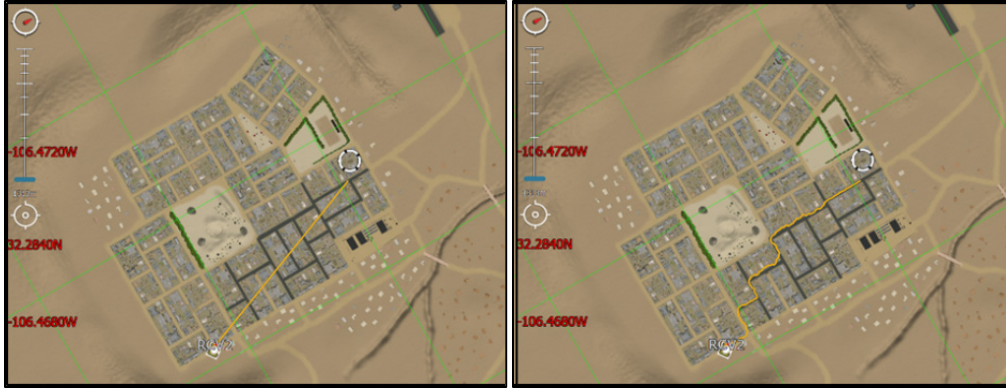
Fig. 1 Route planning using the baseline WMI (left panel) and TRP-equipped WMI (right panel). Routes generated by a single-click supervisory control scheme are shown in yellow. Using the baseline WMI, which merely shows a connection between the origin and destination, it is unclear how the RCV’s local decision-making navigation processes will reach the objective. For example, the vehicle may struggle to navigate entirely within narrow alleys inside city blocks or might even exit and circumvent the city in its entirety, and the baseline WMI does not provide any up-front information for predicting the vehicle’s route. The TRP-equipped WMI, on the other hand, clearly displays the planned route that the vehicle will take, allowing for analysis of the impact of the chosen path, or selection of a new path, during mission planning.
