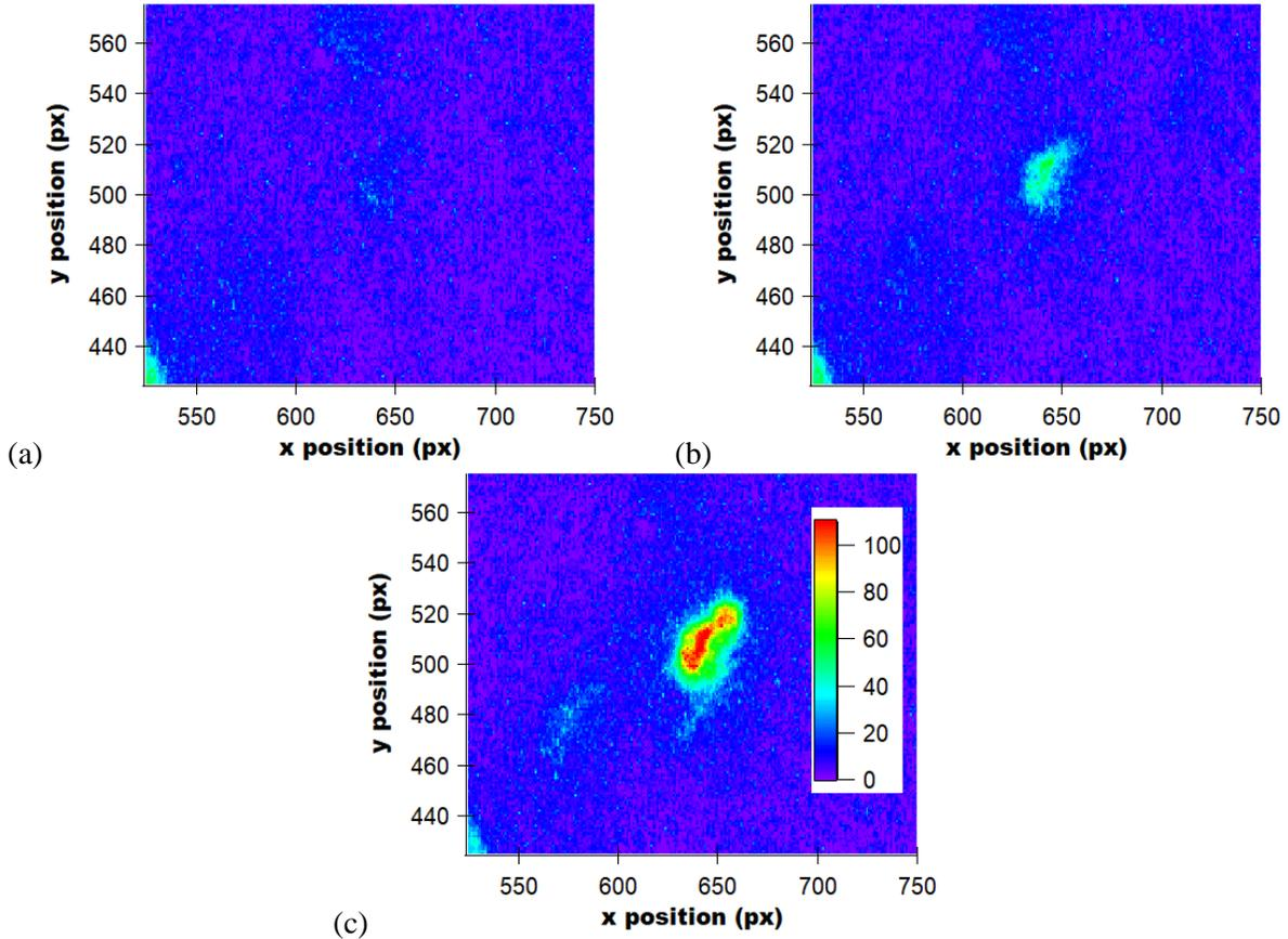
**Figure 8.** Intensity pattern for flat wavefronts (a), a single optimized SLM (b), and two optimized SLMs (c).
