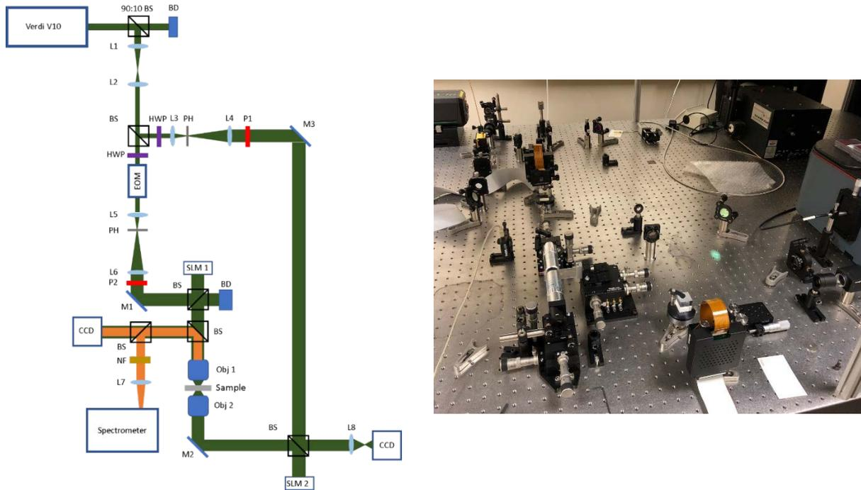
**Figure 10.** Schematic and picture of fully assembled microscope.
