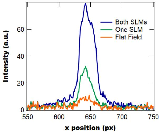
**Figure 9.** Intensity line profile for flat wavefront, single optimized SLM, and two optimized SLMs.
