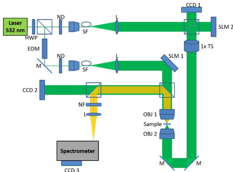
**Figure 1.** Schematic of proposed setup for probing sub-surface reactions via Raman and LIF spectroscopy.
