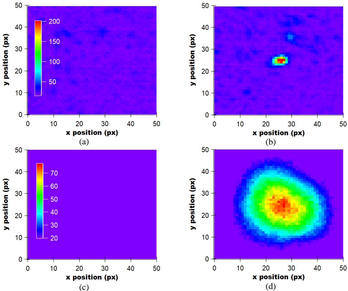
**Figure 2.** Background (a,c) and optimized (b,d) intensity patterns for reflective (a,b) and fluorescence (c,d) feedback.
