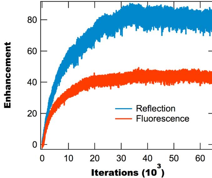
**Figure 3.** Enhancement as a function of iteration for fluorescence and reflective feedback. Optimization was performed using the SGA with 4096 bins.
