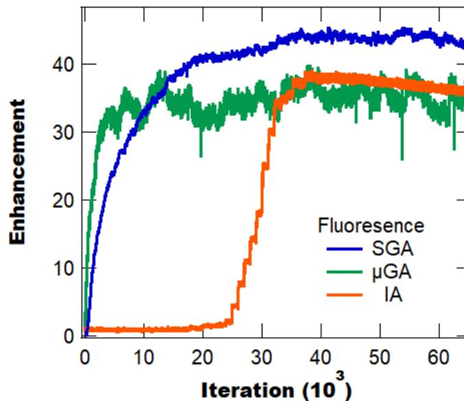
**Figure 4.** Fluorescence enhancement as a function of iteration for three different optimization algorithms and  $N = 4096$  bins.
