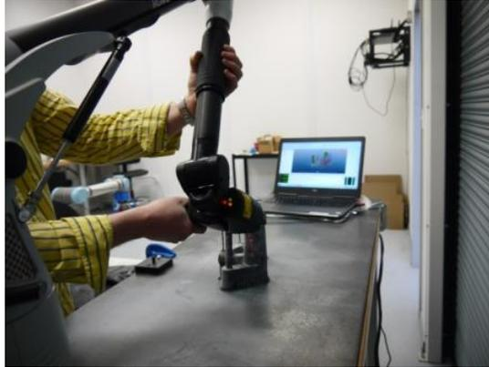
**Figure 4.9.4.** Scanning a distorted swivel link casting tree with the Romer arm scanner
