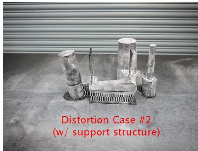
**Figure 3.9.4.** Distorted and scaled 3D polymer printed swivel link casting tree case #2
