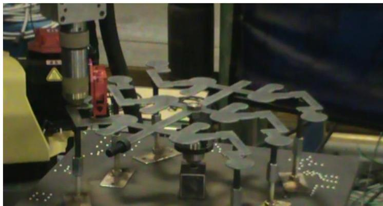
**Figure 4.9.38.** An image of the plasma cutting torch at the first cut location on the casting tree.
