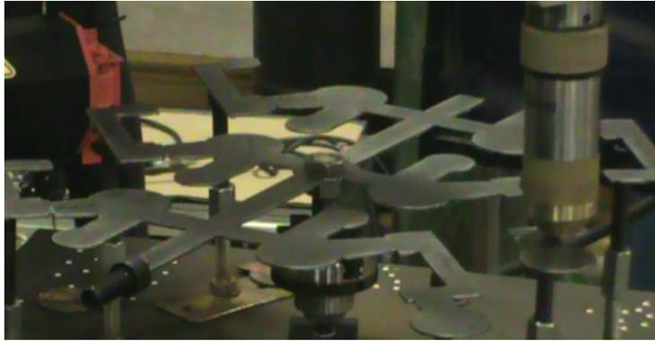
**Figure 4.9.40.** An image of the cutting torch at a subsequent cut location.
