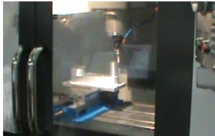
**Figure 4.9.55.** Imaging of probing being performed on Haas mill
