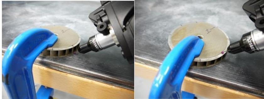
Figure 4.9.65. Images of probing impeller with Romer arm
