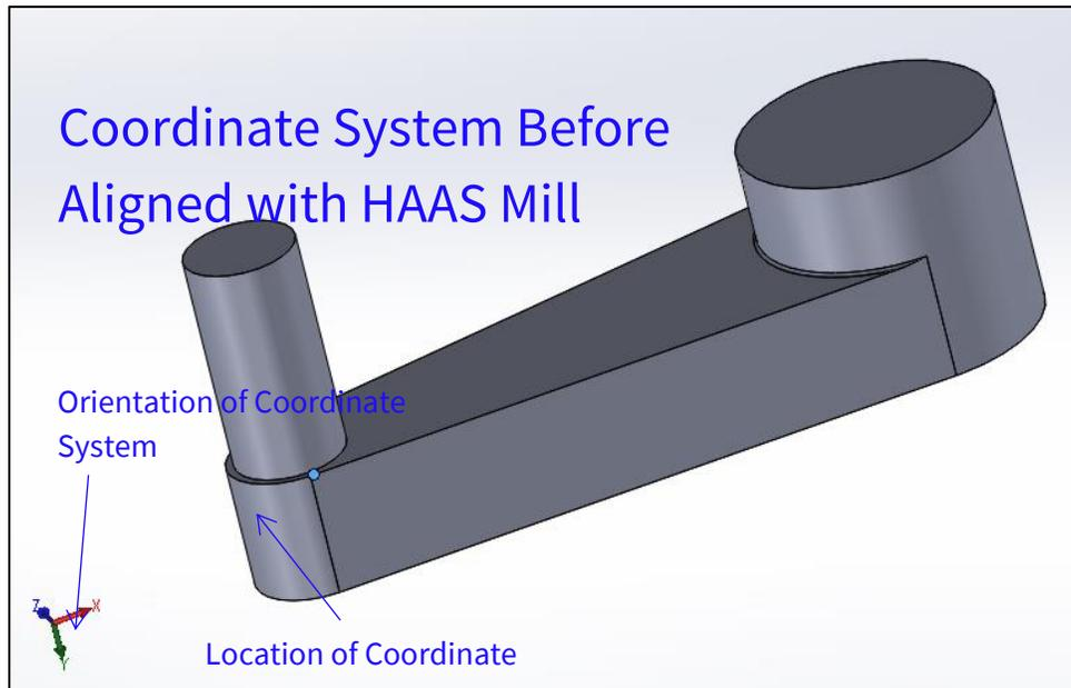
Figure 4.9.53. Image of coordinate system before alignment with Haas mill
