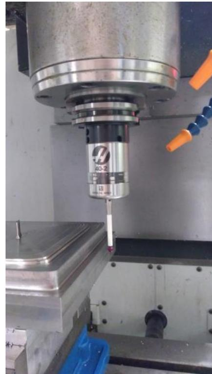
**Figure 4.9.44.** (left) Probe setup in Haas mill at WIU
