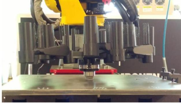
**Figure 4.9.22.** Image of casting tree fixtured through use of a chuck.
