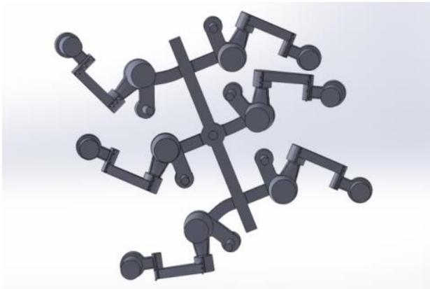
Figure 4.9.12. (left) Top view of casting tree with curved distortion
