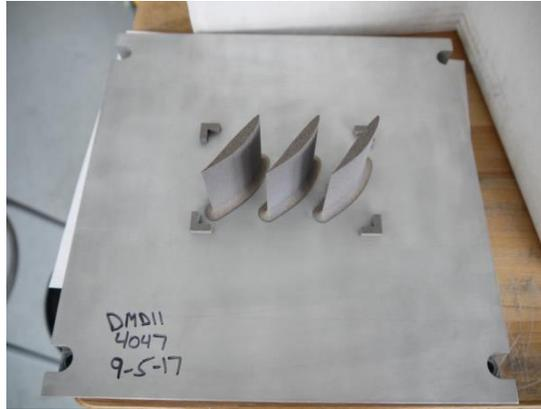
Figure 48. Image of 3D printed aluminum airfoils
