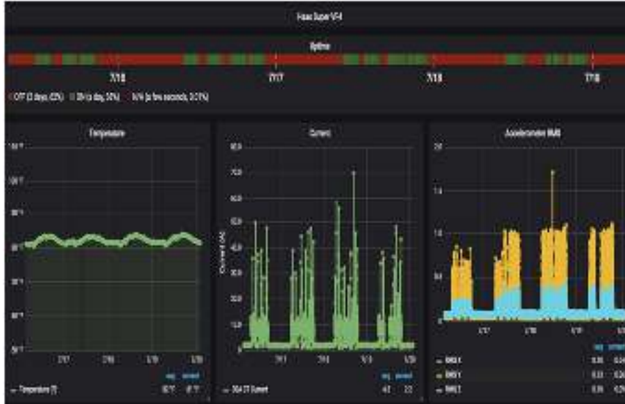
Figure 10-- Sample Milling Application Showing Temperature, Current, and Vibration Data
