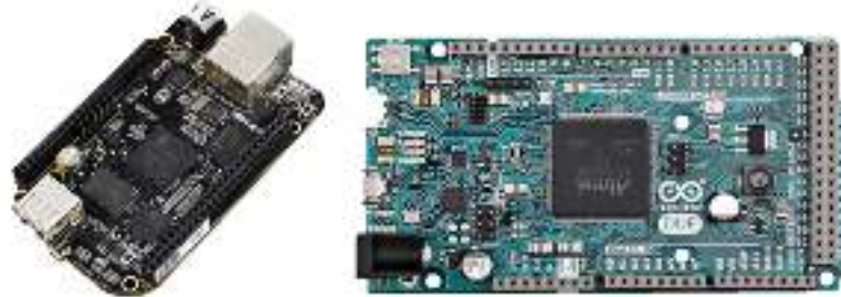
Figure 4-- Prototype Sensor Kits Used BeagleBone and Arduino Processors
