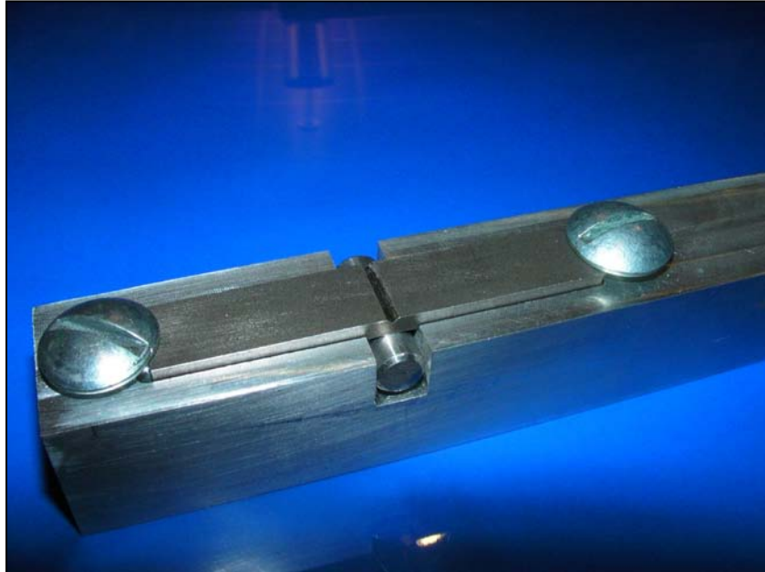
Figure 7. Picture of jig used to deflect the Charpy bar.
