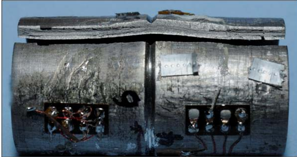
Figure 18. Cylindrical steel cylinder after pressurization test showing longitudinal fracture.
