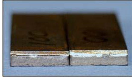
Figure 16a. Non-wetted fracture surfaces (sample number 100-PN).
