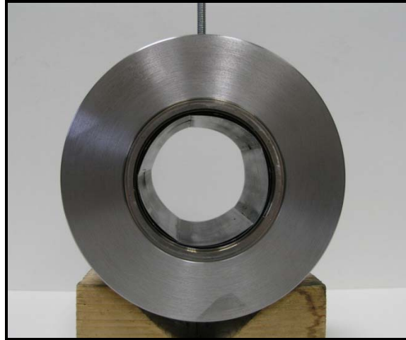
Figure 4. Setup to determine the foil bearing's lift-off speed while supporting 266.9 N.
