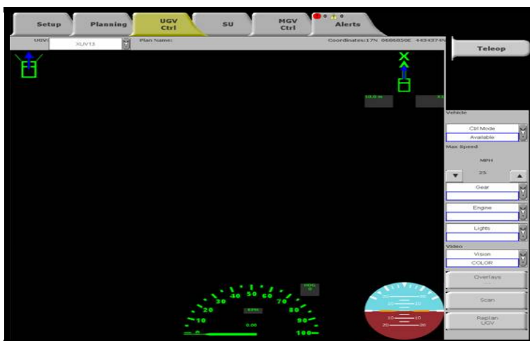
Figure 24. UGV Control – Teleop large portal.
