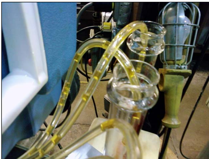
Figure 8. Air in lines at cold temperatures.
