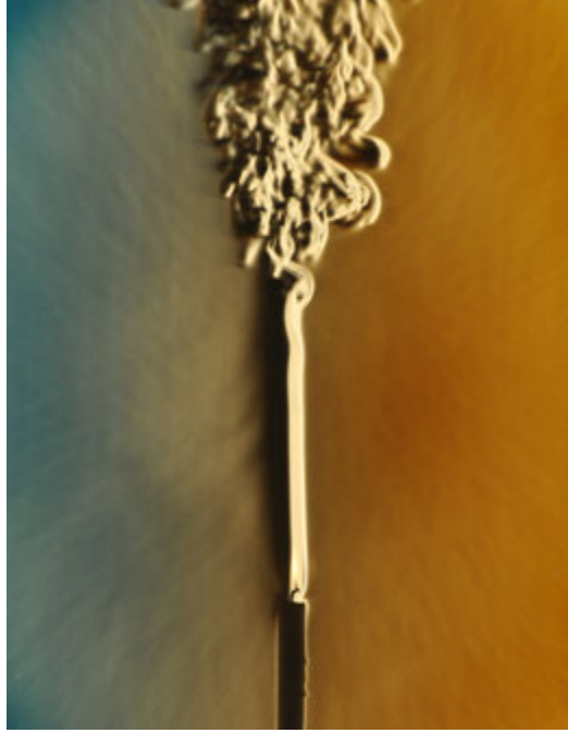
Figure 2: Transition from laminar to turbulent flow above a burning candle. Source: Wikipedia. The Schlieren photograph, created by Dr. Gary Settles of Floviz, Inc. ( http://www.flovizinc.com ), is licensed under the Creative Attribution-ShareAlike 3.0 Unported License.
