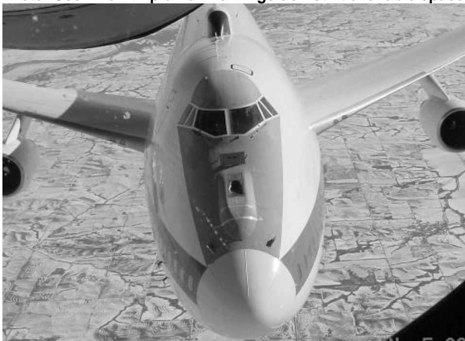
Figure E-6. Two Bar Receptacle Marking
