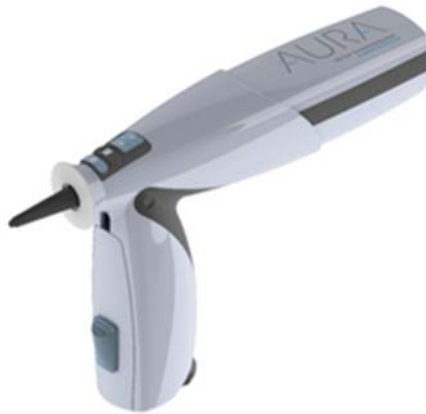
Figure 1. AURA™ 3D ear scanning system by Lantos™ Technologies.
