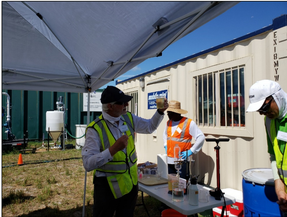
Figure A-6. Demonstration of clumping taking place in algae water immediately after conditioning with coagulant and flocculant.
