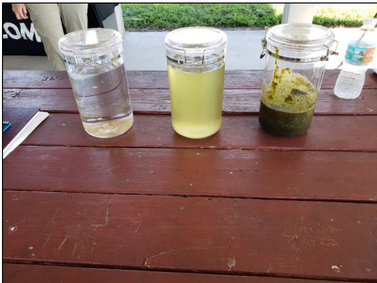
Figure A-18. Display of clarified, processed effluent (left container), algae water collected from the water body (center container), concentrated algal biomass recovered from the liquid-solid separation process (right container).
