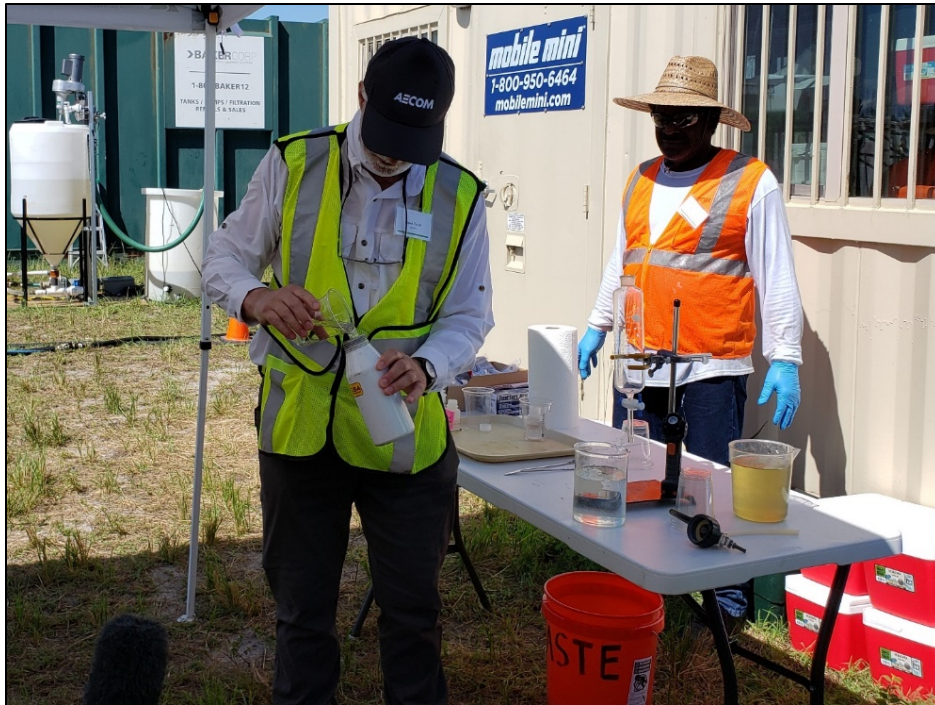
Figure A-4. AECOM liquid-solid separation specialist adding clarified, processed effluent into a container that was subsequently pressurized using a manual air pump.
