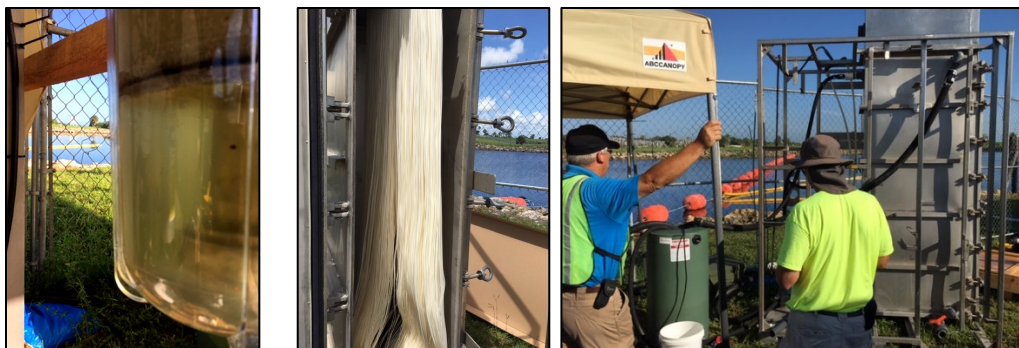
Figure 2-9. Testing of stacked disk filter (left) and ZeeWeed hollow fiber membranes (middle, right) for algae removal at the Moore Haven demonstration site.
