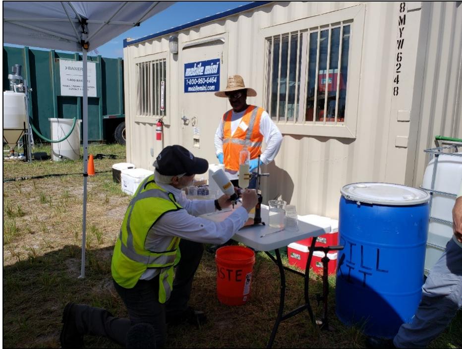
Figure A-10. AECOM specialist opening valve on pressurized vessel to introduce a small stream of microbubbles (white water) into the funnel. The volume of water pressurized was 25% of the volume of algae water being treated.
