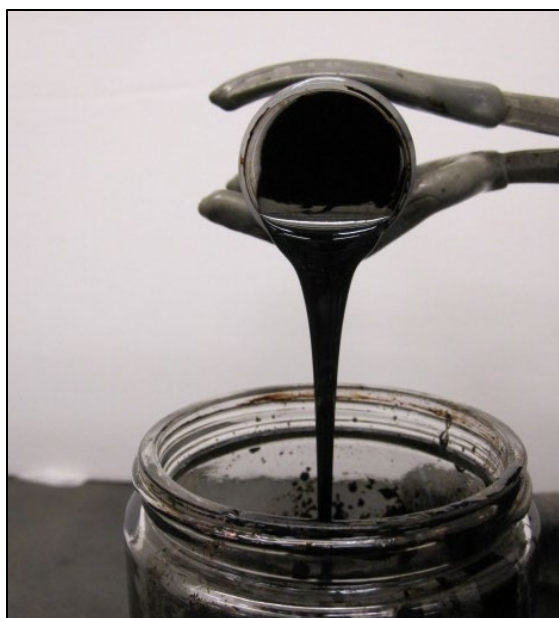
Figure 3-12. Biocrude oil generated via Hydrothermal Liquefaction at PNNL using the concentrated algae biomass collected from the treatment demonstration in Moore Haven, FL.
