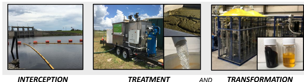
Figure 1-1. Overview of the three key steps in the HABITATS approach for intercepting, treating, and transforming algae-laden waters.
