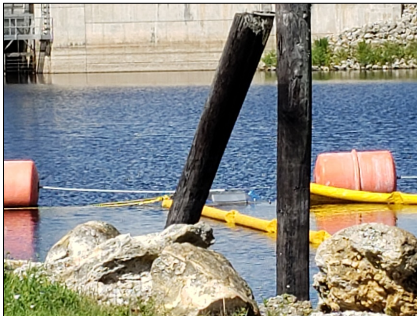
Figure A-2. Weir skimmer (silver box) positioned at opening of boom weirs.
