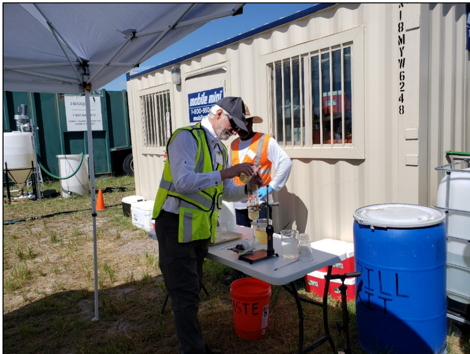
Figure A-9. AECOM specialist adding conditioned algae water into separatory funnel.
