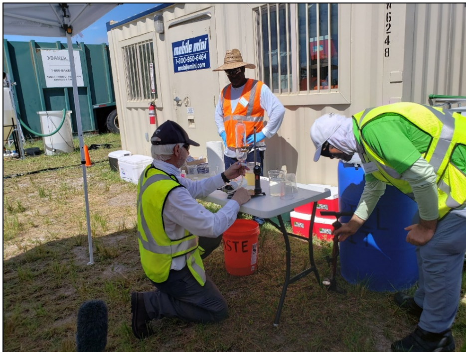
Figure A-8. AECOM specialist attaching tube from pressurized vessel containing clarified effluent to a separatory funnel before the separation process.
