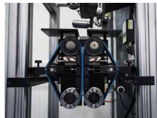
Counterclockwise from top left, Lauren Cantley, a postdoctoral associate in the Chemical, Microsystem, and Nanoscale Technologies Group, adjusts the gauge near the top of the fiber draw tower as it pulls a fiber. The roller guides below the tower keep the fiber straight before it is spooled. Knitting machines weave the fibers into textiles and garments.
