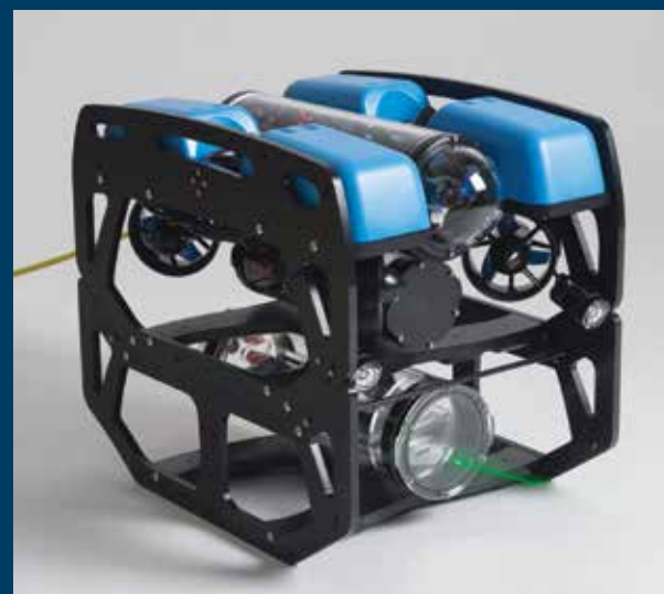
In 2017, optical communication terminals were integrated onto Blue Robotics' remotely operated underwater vehicle, the BlueROV2 platform, above, for in-ocean demonstrations.
