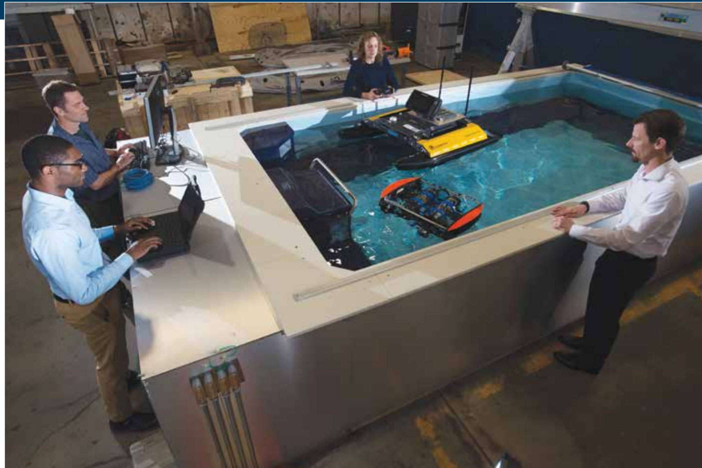
The Laboratory is developing advanced technology for unmanned undersea and surface vehicles. This Maritime Autonomy Test Tank is a controlled environment in which staff can refine capabilities in autonomy, sensing, signal processing, and communications prior to open-water demonstrations.
