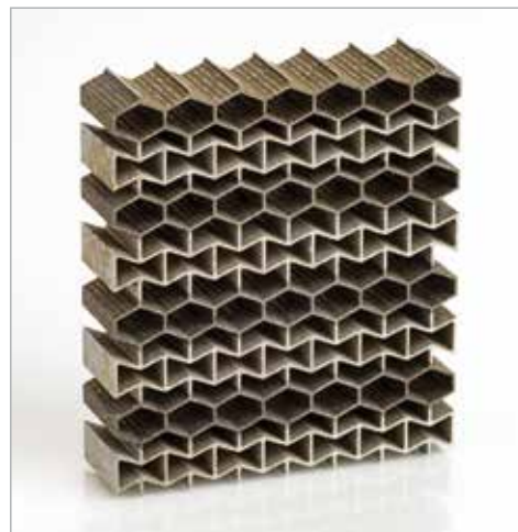
This photograph of a prototype of zero thermal expansion metal manufactured with ultrasonic consolidation and electric discharge machining shows the titanium hexagonal cells and the aluminum re-entrant or "bow tie" cells. This sample measures about 1 inch square.
