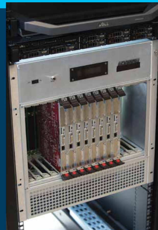
Shown above is a 64-node version of the graph processor. This system has similar processing performance to today's best supercomputers but consumes only 1/100th of the power.
