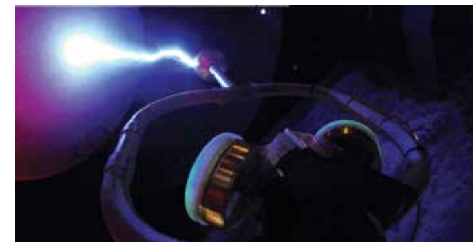
The prototype BEACON instrument takes a near strike from the Van de Graaff generator at the Boston Museum of Science. Testing in the museum's Theater of Electricity allowed the BEACON team to simulate some of the extreme electrical environments that the instrument may experience while mapping the charge structure of a cloud.
