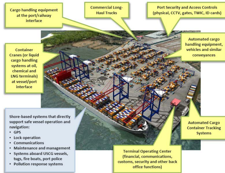
Figure 1: Typical Shore-based, Maritime Transportation Industrial Control Systems 16
