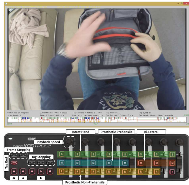
Figure 6: A screenshot from the custom video player software (top). Logged tags are shown in the playback progress bar. A hardware midi interface (below) is used to precisely control video playback and tagging.
